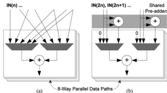
Figure 4. Correlator designs for a packet synchronizer. (a) Wide-input multiplexer based design. (b) Shared pre-adder-based design.
