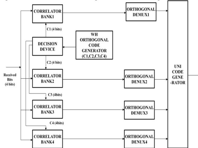
Fig.7. Biorthogonal decoder.
