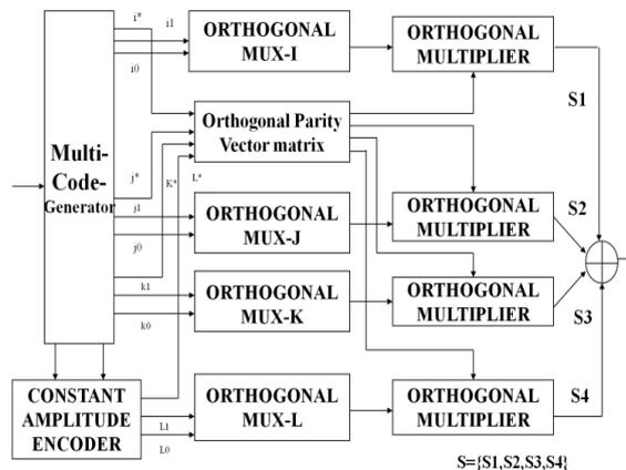
Figure 2. Biorthogonal Encoder
