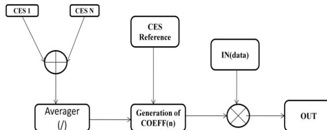
Fig.6. Channel equalizer structure.
