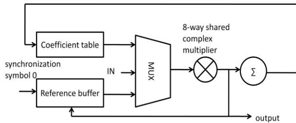
Figure.5. CFO compensator structure.
