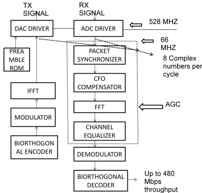
Fig 1: Overall architecture of MB-OFDM baseband to use 8-way parallel data-paths.
