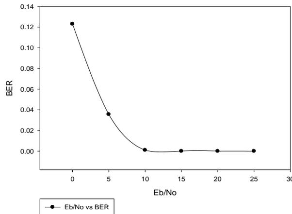
Figure 9. SNR vs BER of proposed system.
