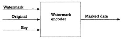
Figure 3.1: Generic Watermark Embedding Scheme The output of the embedding process is always the watermarked data/image
