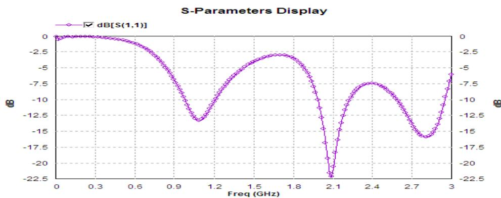
Fig. 2 Return Loss Curve of the Designed Antenna Structure
