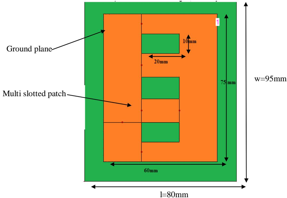
Fig.1 Design of multi slotted Microstrip Patch Antenna
