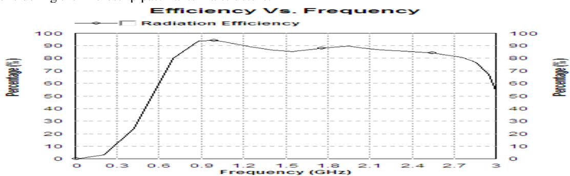
**Fig. 7** Radiation Efficiency
