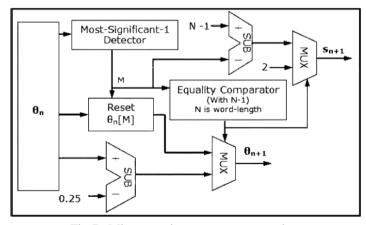
Fig 7. Micro-rotation sequence generation.
