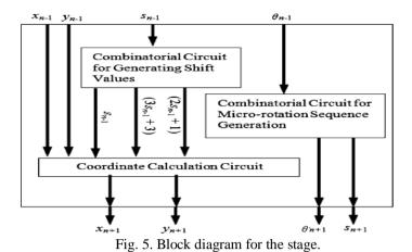
The combinatorial circuit for generating the micro-rotation sequence is shown in Fig. 4. The number of iterations required in a CORDIC processor decides the rollover count of the counter. The rollover count is seven for basic shift =2 and ten for basic-shift =3.
