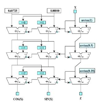
Fig.2. Parallel/Cascaded CORDIC
