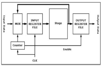
Fig.4. Recursive architecture of the proposed CORDIC processor.
