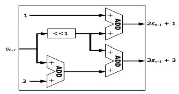
Fig. 6. Combinatorial circuit for generating the shift values.
