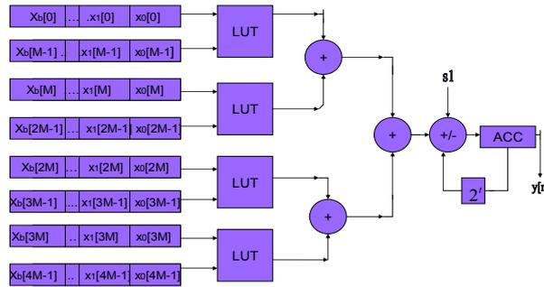
**Figure 3.1 DISTRIBUTED ARITHMETIC WITH 4-INPUT LOOK UP TABLE**
