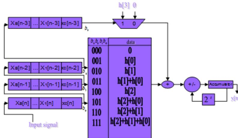
**Figure 2.2.2(a):** Proposed DA architecture for a 4-tap filter ( $2^3$  word LUT implementation of DA)
