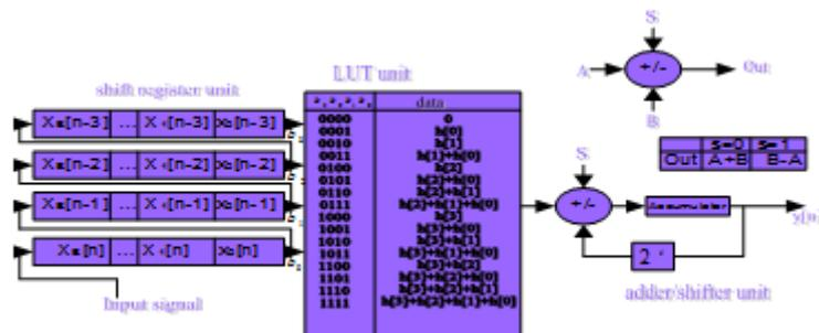
Figure 2.1: Original LUT-based DA implementation of a 4-tap filter
