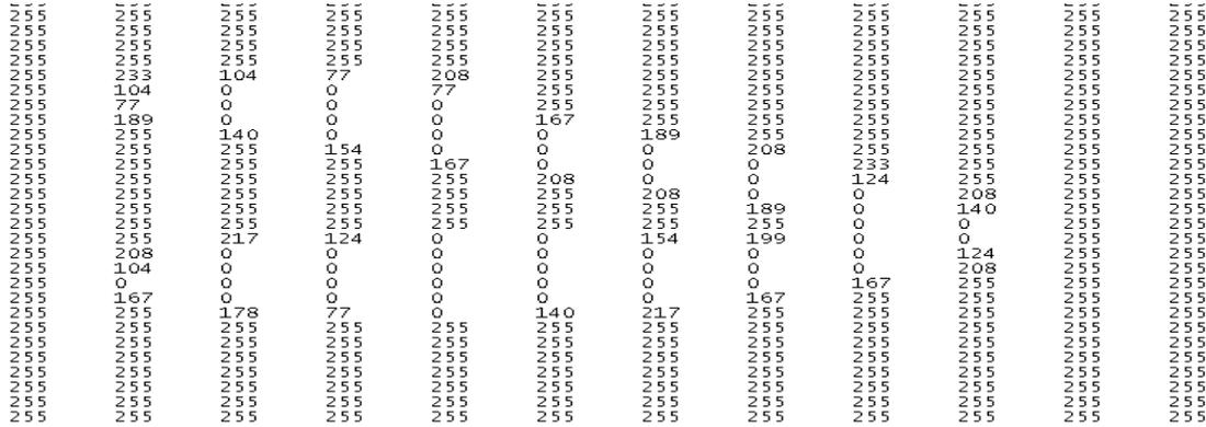
Fig.- 7: An M by N array for the image of Bangla digit one (১)
