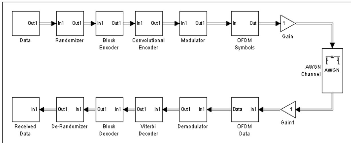
Fig 2 Simulink model of IEEE 802.16e
