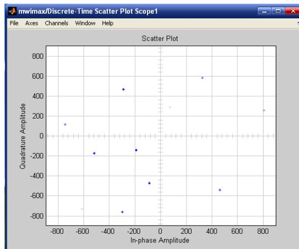
Fig 4 Scatter Plot for 4-QAM
