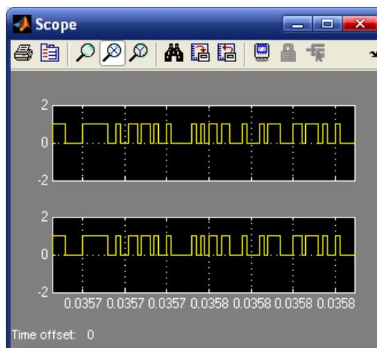
Fig 3 Transmitted and Recovered Information Signals
