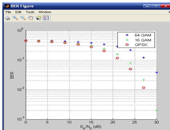
Fig 5 BER vs.  $E_b/N_0$  Graphs for different modulation schemes
