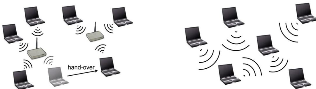
Fig. 1(a) an infrastructure network with two base stations.
