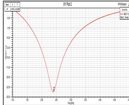
Figure 3: Result showing  $f_r$  vs. S11
