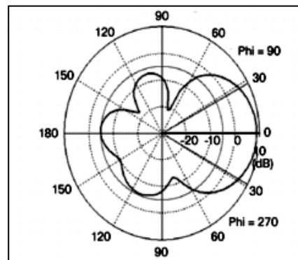
Figure 5: Elevation plane pattern on FR4
