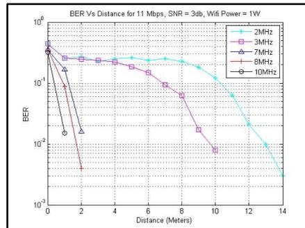
**Figure 2b:** Simulated BER performances for different offset frequencies with distance variation. The graph shows that the BER increases exponentially with offset frequency increment.
