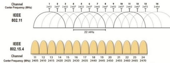
**Figure 1:** Zigbee and WLAN channels in 2.4 GHz band[12]
