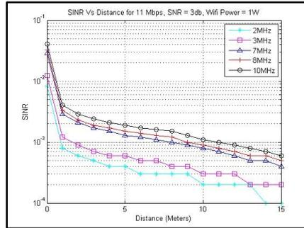
**Figure 2a:** Simulated SINR performances for different offset frequencies with varying distance, the graph shows that offset improves the SINR by 10 times when offset increased from 2 to 10 Mhz for every value of distance.
