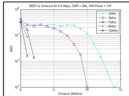
**Figure 4b:** Simulated BER performances for different offset frequencies with distance variation. The graph shows that the BER decreases exponentially with offset frequency increment.
