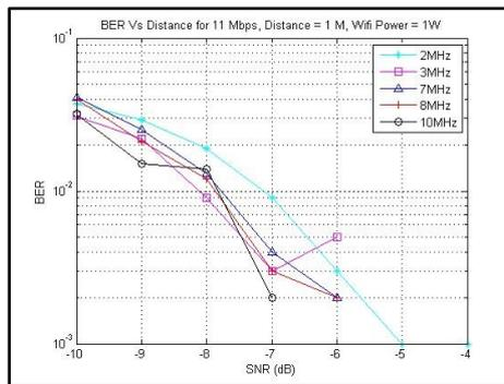
**Figure 3:** Simulated BER performances for different offset frequencies with varying AWGN. The offset variation doesn't affect the BER variation (overlapping graphs). The variation in BER is due to SINR only.
