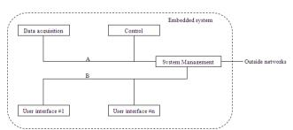
Fig. 1.Example embedded system based wireless node architecture
