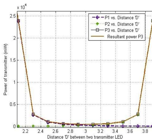
Figure7. Degradation in received power with distance 'D'(meter). P1 and P2 are the transmitter LED power.
