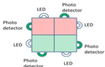
Figure 1 Top view of Transceiver section
