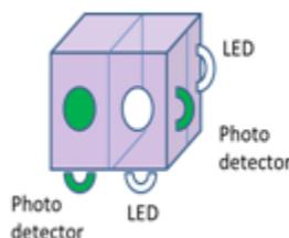
Figure 2 Side view of Transceiver section
