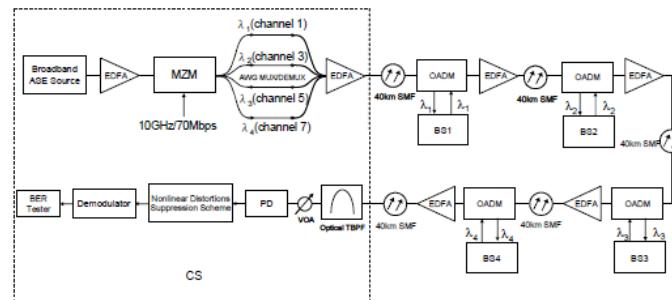
Fig.2. Experimental configuration of our proposed full-duplex ROF transport systems.
