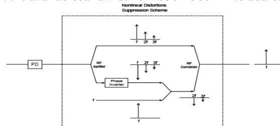
Fig. 3. Functional diagram of the nonlinear distortion suppression scheme.
