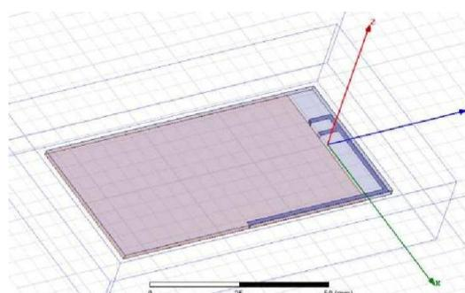
Fig 3: PIFA-L ANTENNA MODEL
