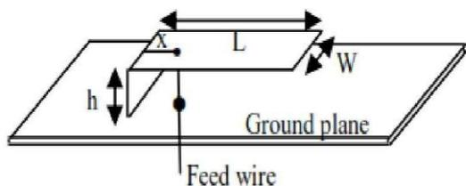
Fig 1: The Planar Inverted-F Antenna (PIFA).
