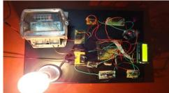
Stage 2: The meter detects the number of pulse consumed by the load and display on the LCD.
