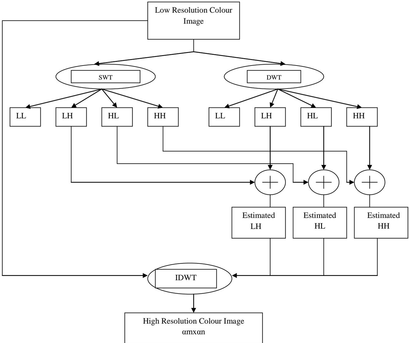
Fig.3 Block Diagram DWT and SWT based Image Resolution Enhancement
