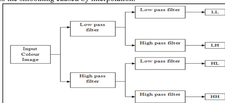
**Fig.2 Block diagram of SWT Filter Banks of level.1**
