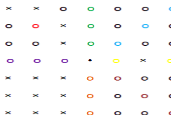
Fig 3. Considered pixels in directional median inpainting, \circ shows a known pixel, \times shows an unknown pixel, color pixels show considered pixel in different directions.
