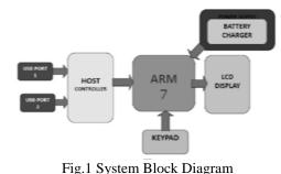
ARM (LPC 2138): It is the heart of the system. It is important unit of the system because it reads data which we programmed and stored into its ROM,
