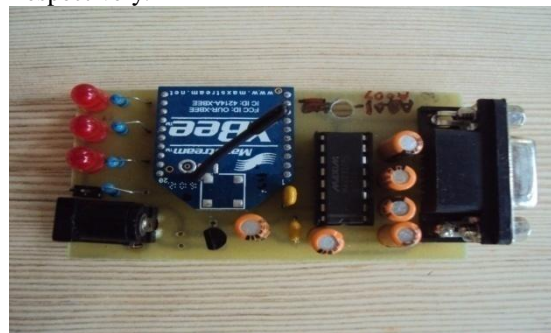
Fig.7 Master node/Monitoring Node
