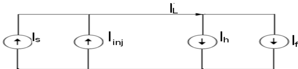
Fig:4 Basic Operating Principle of SAPF
