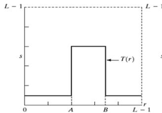
Figure 6. Range [A, B] of grey levels by reducing all others to a constant level.
