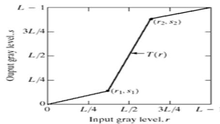
Figure 3. Various degrees of grey levels at output and their affects on contrast.
