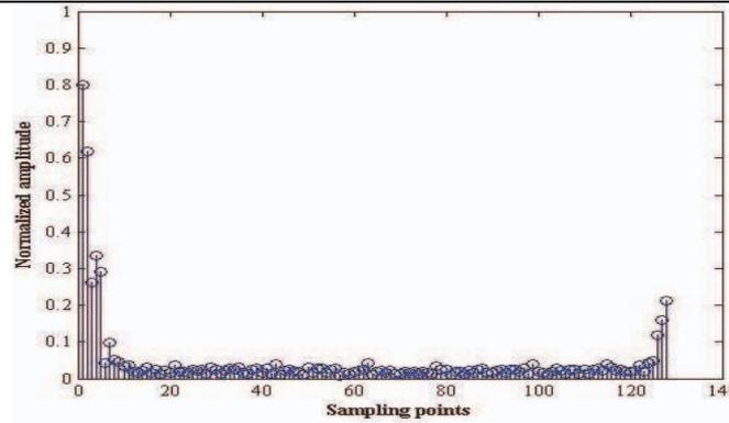
Figure 1. The channel impulse response in non-sample-spaced channel
