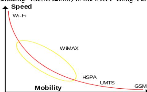
Speed vs. mobility of wireless systems: Wi-Fi, High Speed Packet Access (HSPA), Universal Mobile Telecommunications System (UMTS), and GSM
