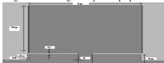
Fig. 1.1 Geometry of proposed antenna
