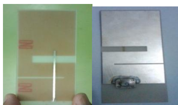
Fig 7. Shown Fabricated Antenna Had Been Through Etching Process.
