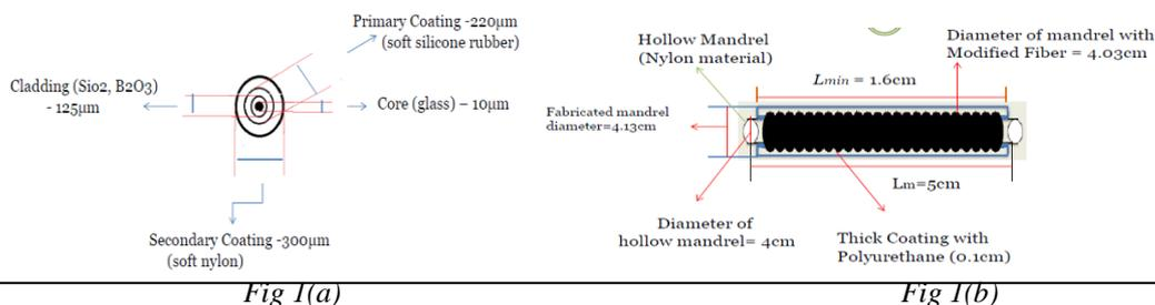
The molding layer is assumed to be only coated on the fiber layer and has a thickness of less than 1mm. Assuming that the fiber sensor response is driven solely by the mandrel response, it is clear that a Circumferential change in the mandrel couples directly to a length change in the fiber. The phase of light propagating through an optical fiber is defined as,
