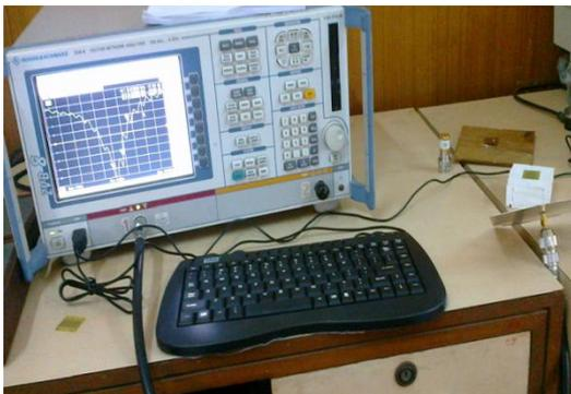
Fig.4-Photograph of fabricated microstrip antenna.
