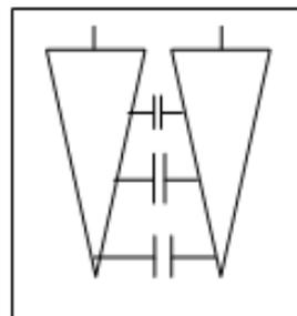
**Fig.3-conical electrode Shape capacitor**
