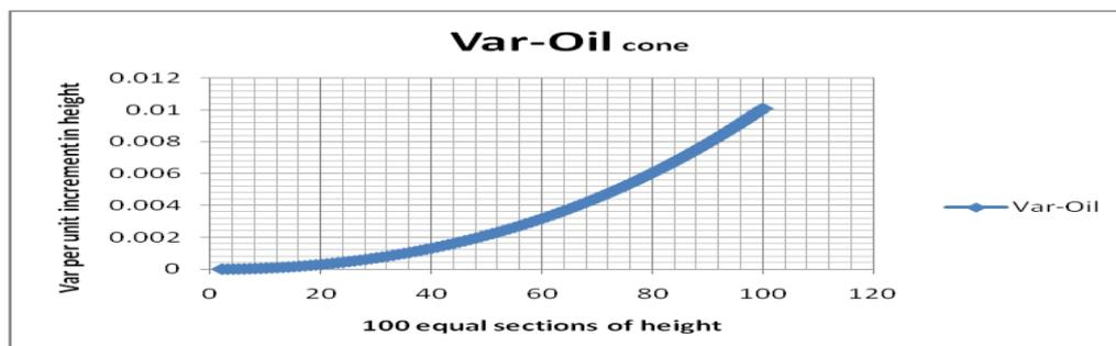
Fig. 14- VAR compensation by conical electrode.
