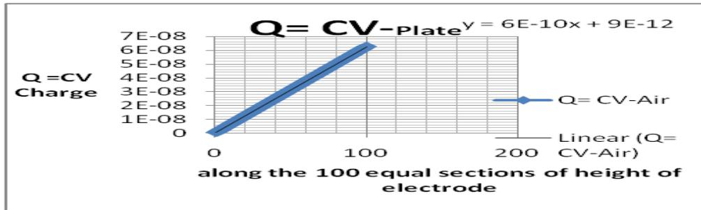
Fig.10- charge distribution with parallel plate capacitor.
