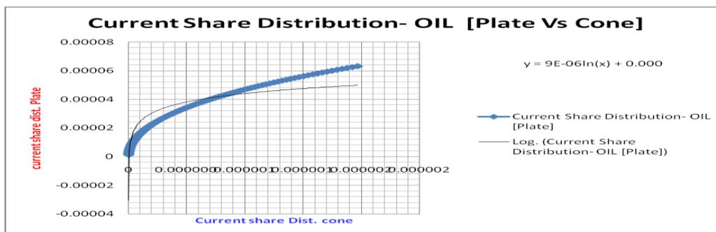
Fig.12- Relationship between current shares of both capacitor types.
