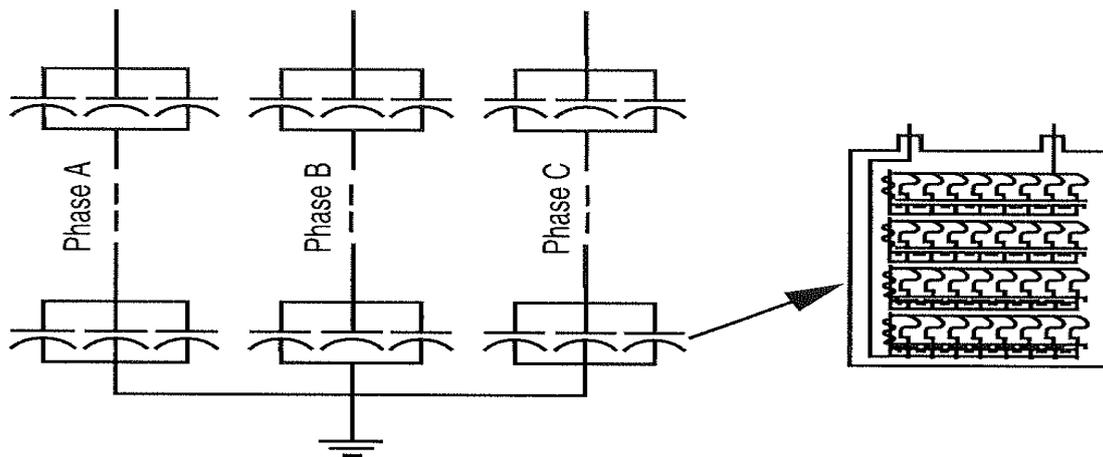
**Fig.1-capacitor banks in industry having puncturing of electrode problem**
