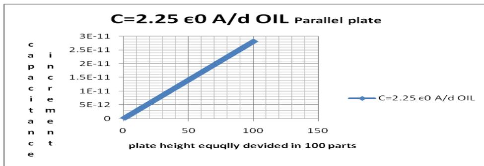
Fig.5 capacitance development in parallel plates-oil
