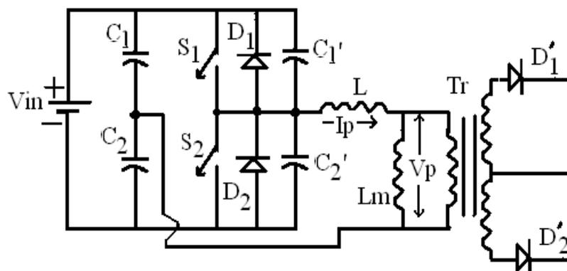
Fig.1 Half bridge ZVS-Clamped voltage configuration
