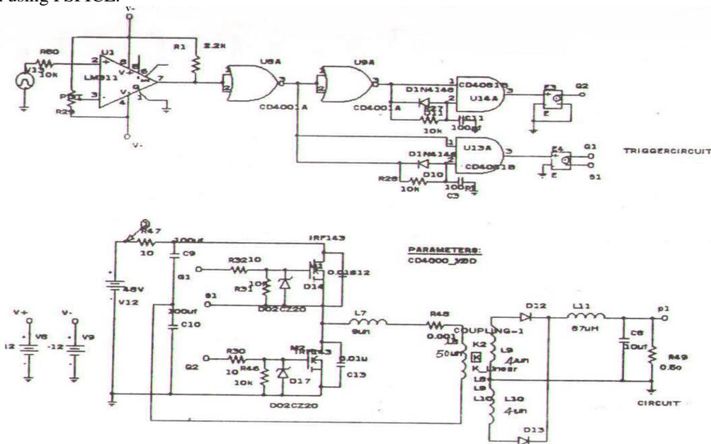
Fig.6. Triggering and Power circuit in PSPICE
