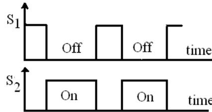
Fig.2 Gate pulse for APWM control
