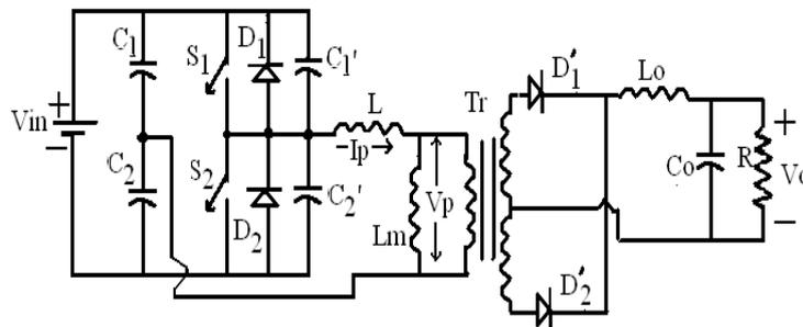
Fig.3 Half bridge LC filter circuit
