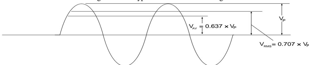
**Fig 8: Measuring sinusoidal alternating current**
