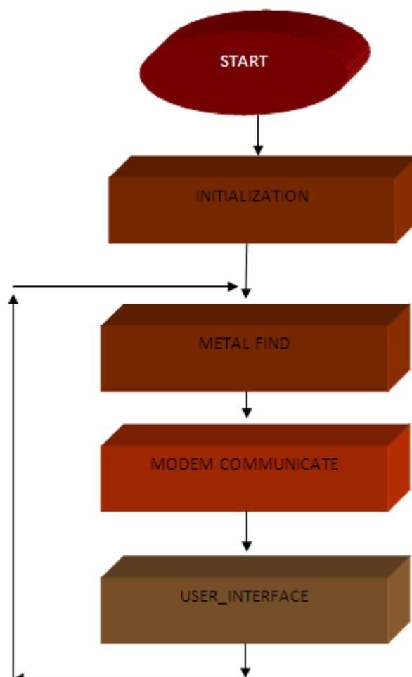
Fig 9: Flow Chart for the Main Software
