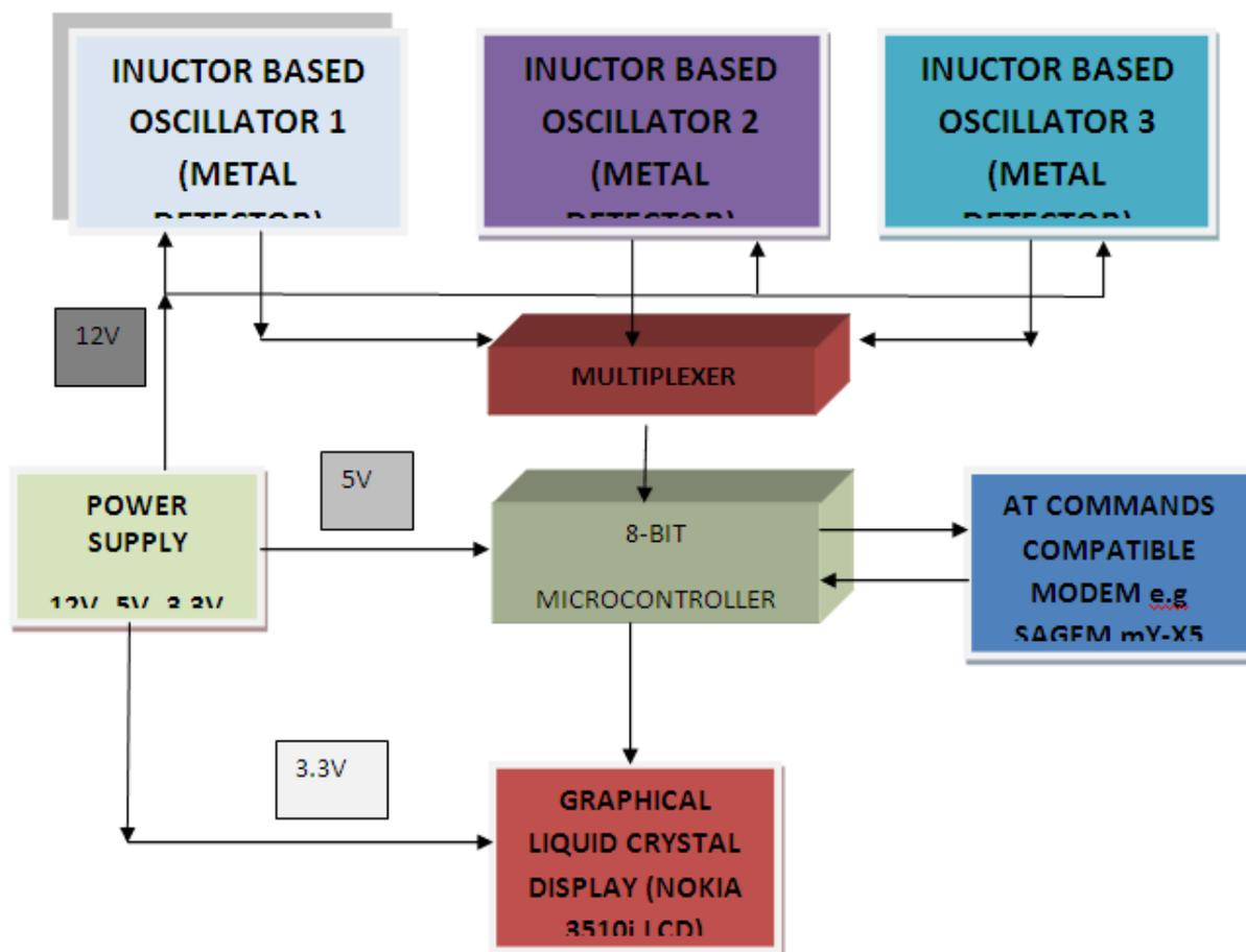
Fig 1: Block Diagram of the Hardware
