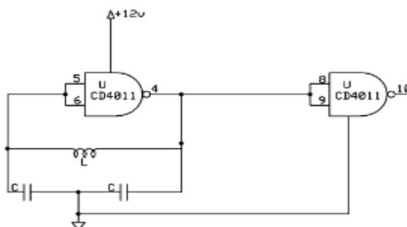
Fig 2: Metal Detector Schematic
