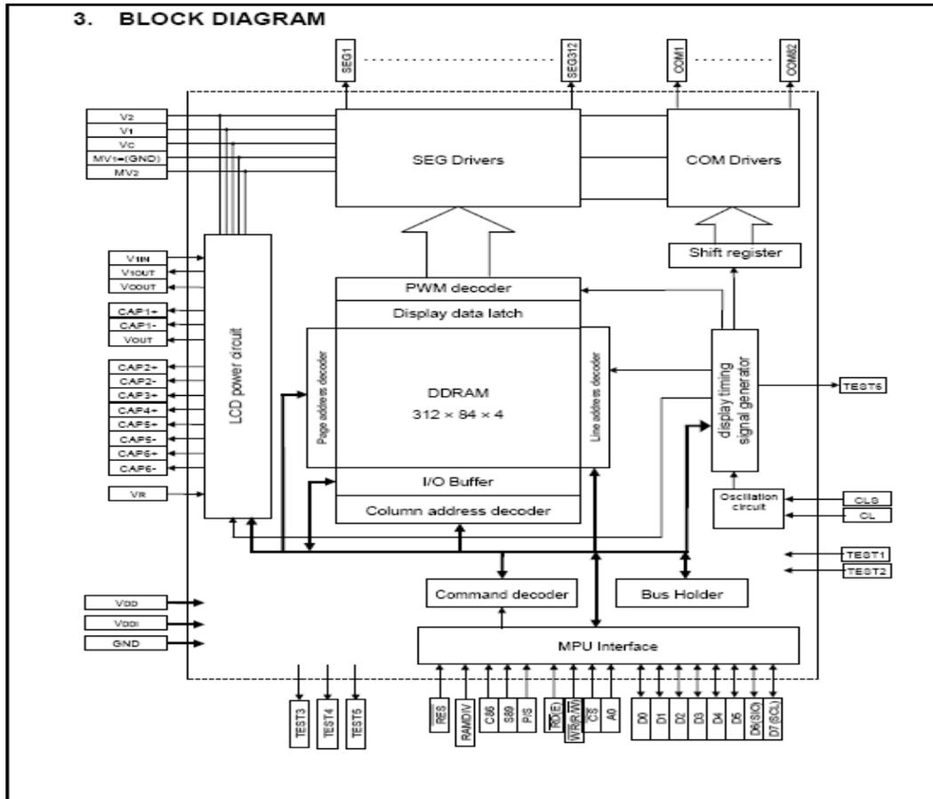
Fig 3: Block Diagram of GLCD
