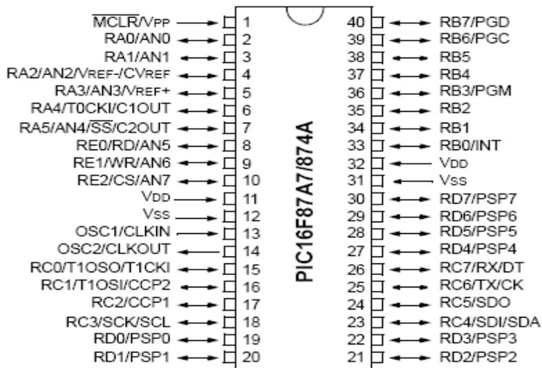
Fig 4: Pin Diagram of the Microcontroller
