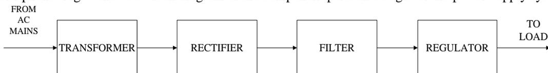
Fig 7: Block Diagram of Power Supply Unit
