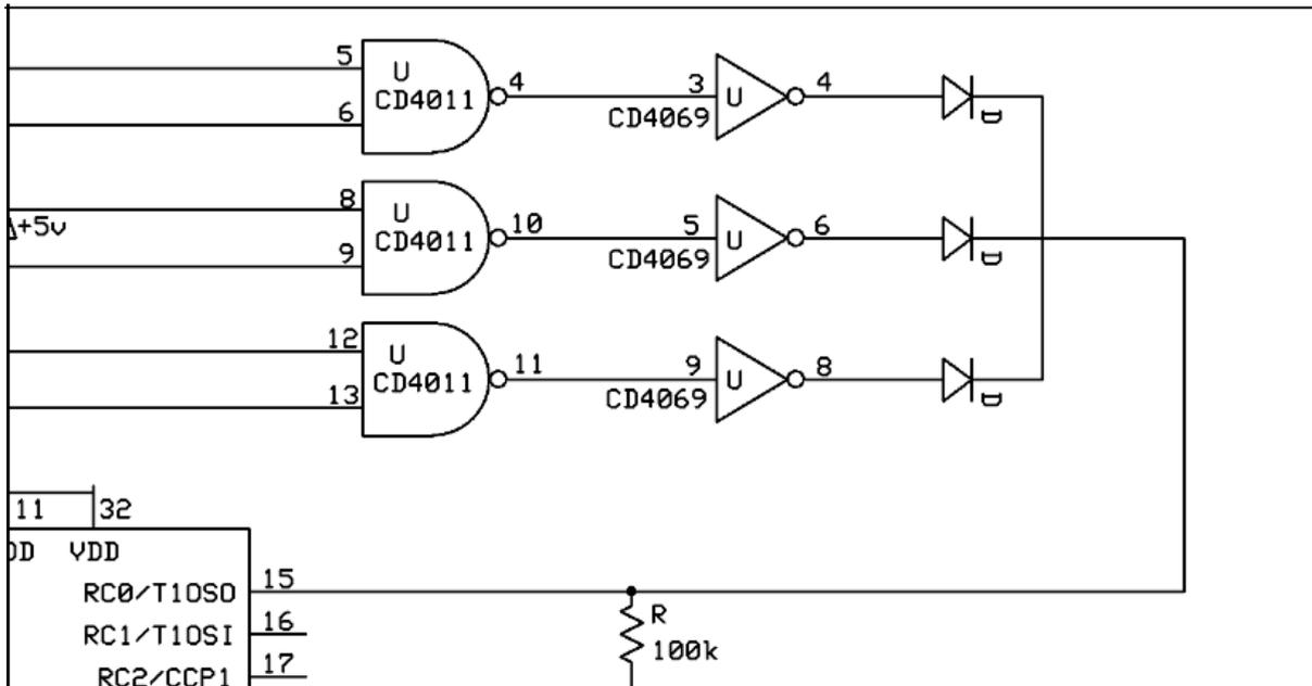
Fig 5: Diagram of Multiplexer with Three Channels
