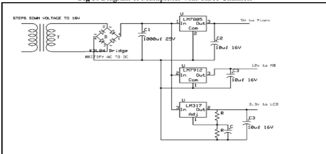
Fig 6: Circuit Diagram of the Power Supply Unit
