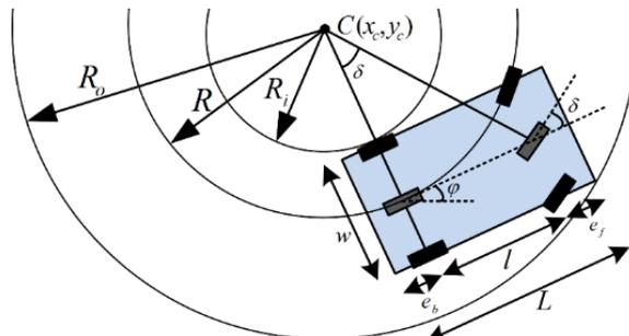
**Fig. 4** geometry of a vehicle turning with a constant steering angle  $\delta$
