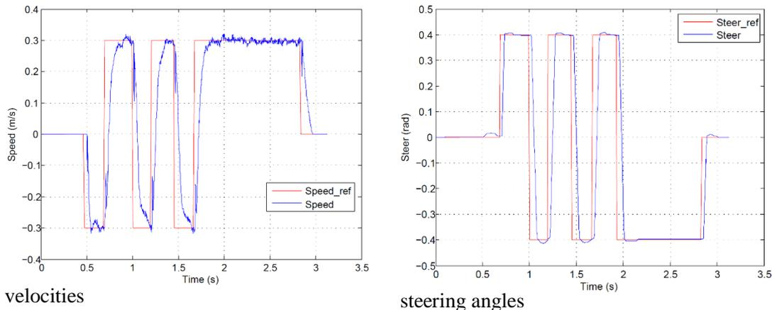
Fig. 12 vehicle and reference velocities and steering angles
