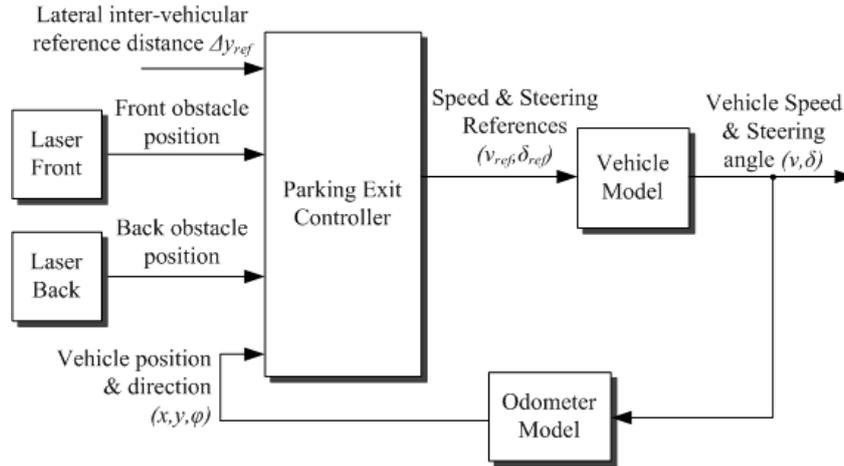
**Fig. 3** functional Structure of Parking Exit Controller
