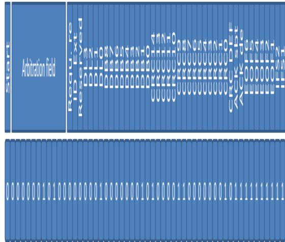
Figure 3 CAN standard frame
