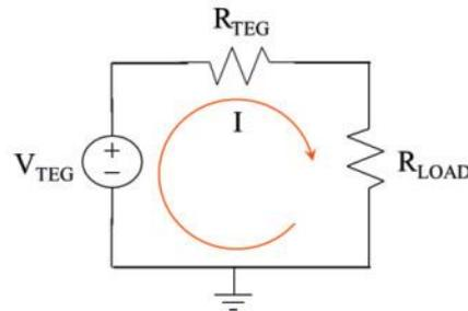
Fig 4(b) -Thevenin equivalent circuit of solar TEG [14]
