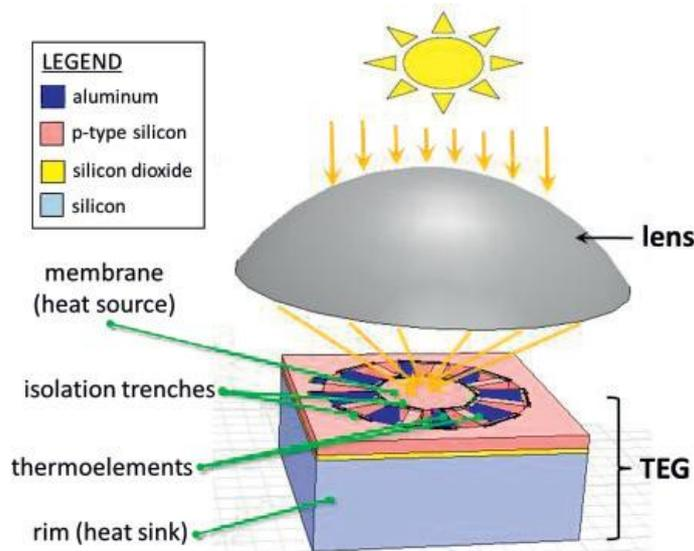
Fig 3- Solar TEG with a lens concentrating solar radiation onto the device [14]
