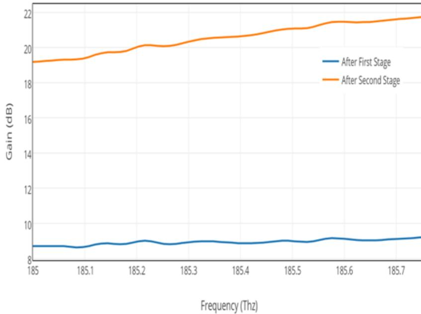
**Fig.2** Gain at First and Second stage of HOA
