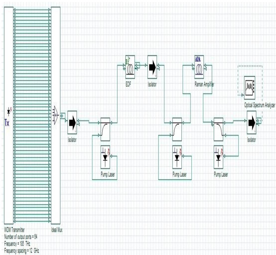
**Fig 1** Simulation Setup of 64×20Gbps HOA System.
