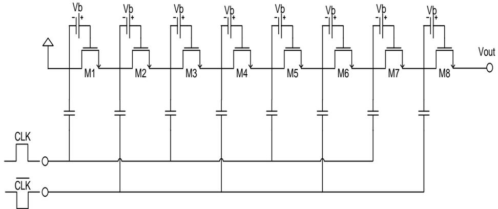
**Fig.1** Schematic of an eight-stage NMOS charge pump using external  $V_{th}$  cancellation (Bodies of all transistors are connected to ground.)
