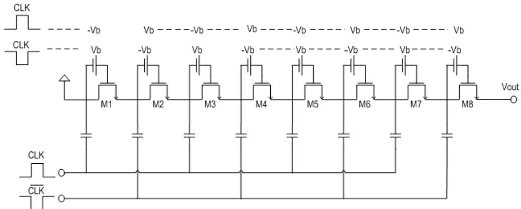
**Fig. 3** Schematic of an eight-stage NMOS charge pump using enhanced external  $V_{th}$  cancellation. (Bodies of all transistors are connected to ground.)
