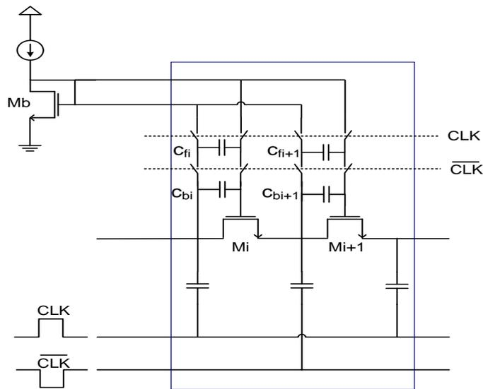
**Fig. 2** Implementation of external  $V_{th}$  cancellation (EVC) technique.
