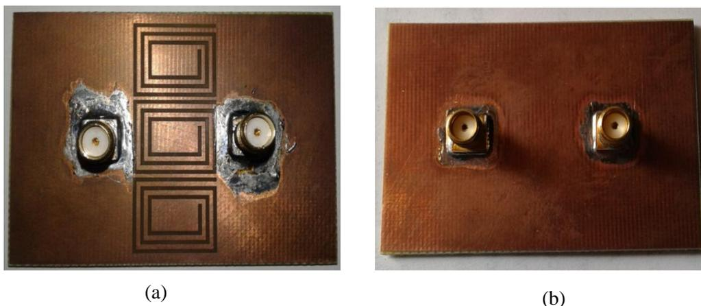
Figure 10. The photo of the bottom view, (a) with solid ground “without CSSRs” and (b) with CSSRs etched in the ground plane.
