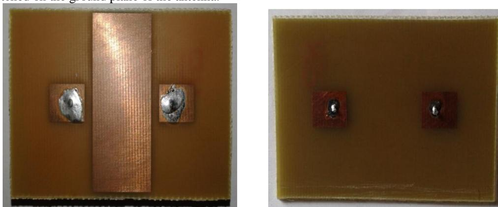
Figure 9. The photograph prototype of the top view, (a) without floating ground and (b) with floating ground.
