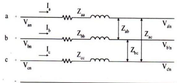
**Figure 1 Channel Model Three Phase**
