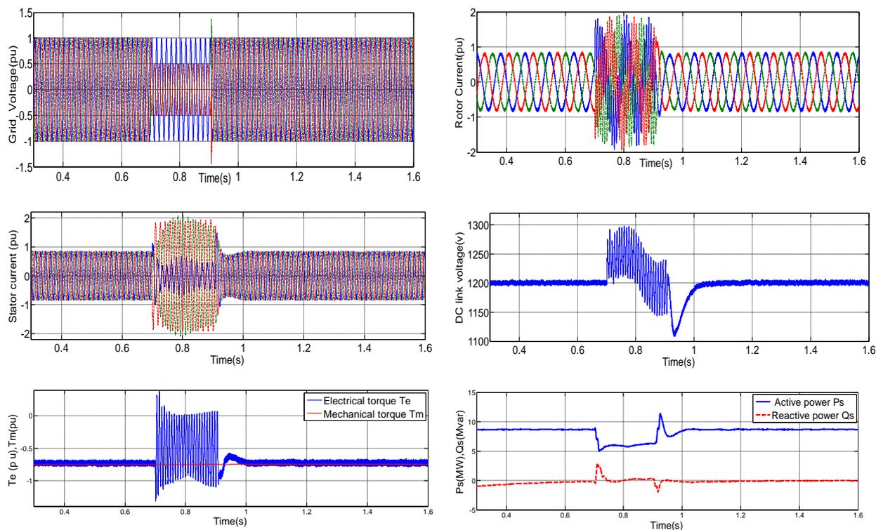
**Fig. 4: Phase b to c short circuit for 0.2**
