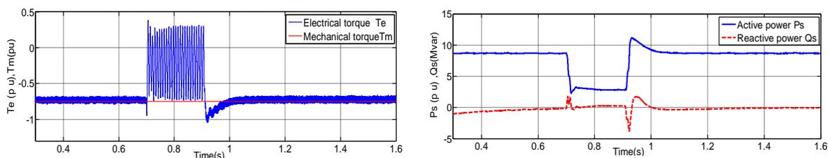
Fig. 10: Phase *b* to *c* short circuit for 0.2s with Crowbar and a DC-chopper protection scheme
