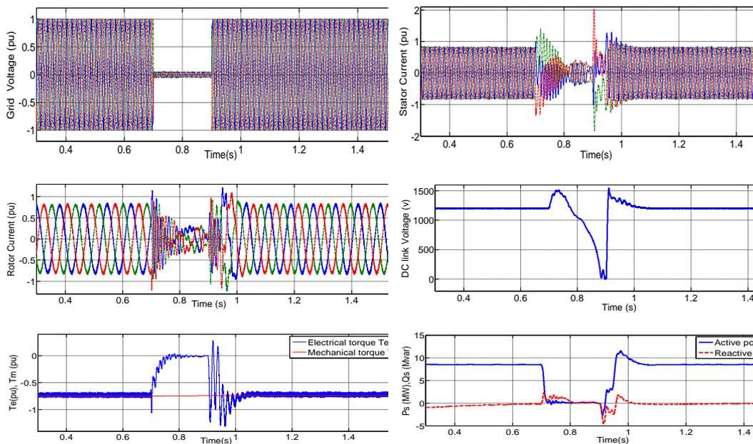
Fig.6: Three-phase 0.95pu voltage dip for 0.2s with Series Resistor protection scheme
