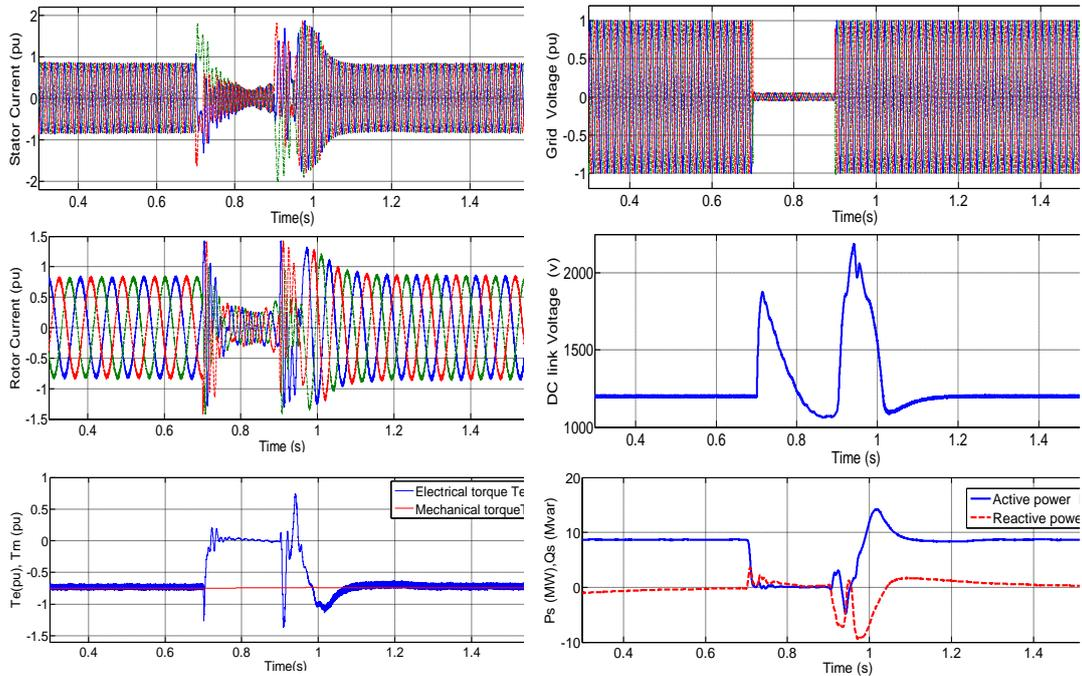
**Fig. 9: Three-phase 0.95pu voltage dip for 0.2s with Crowbar and a DC-chopper protection scheme**
