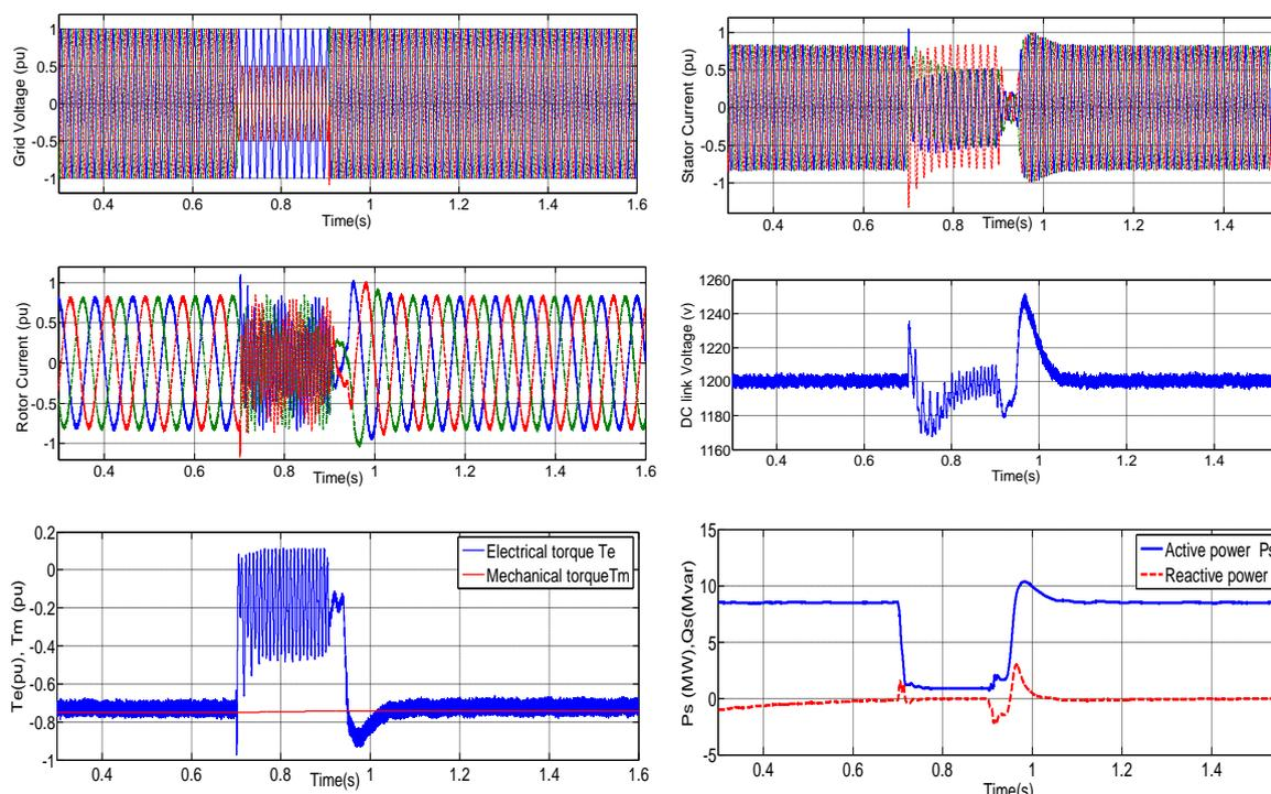
**Fig. 7: Phase b to c short circuit for 0.2s with Series Resistor protection**
