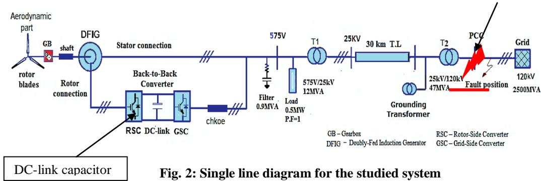
Fig. 2: Single line diagram for the studied system
