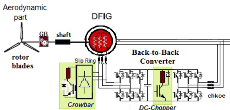
**Fig. 8: DFIG based system extended by Crowbar and DC-chopper Protection scheme**
