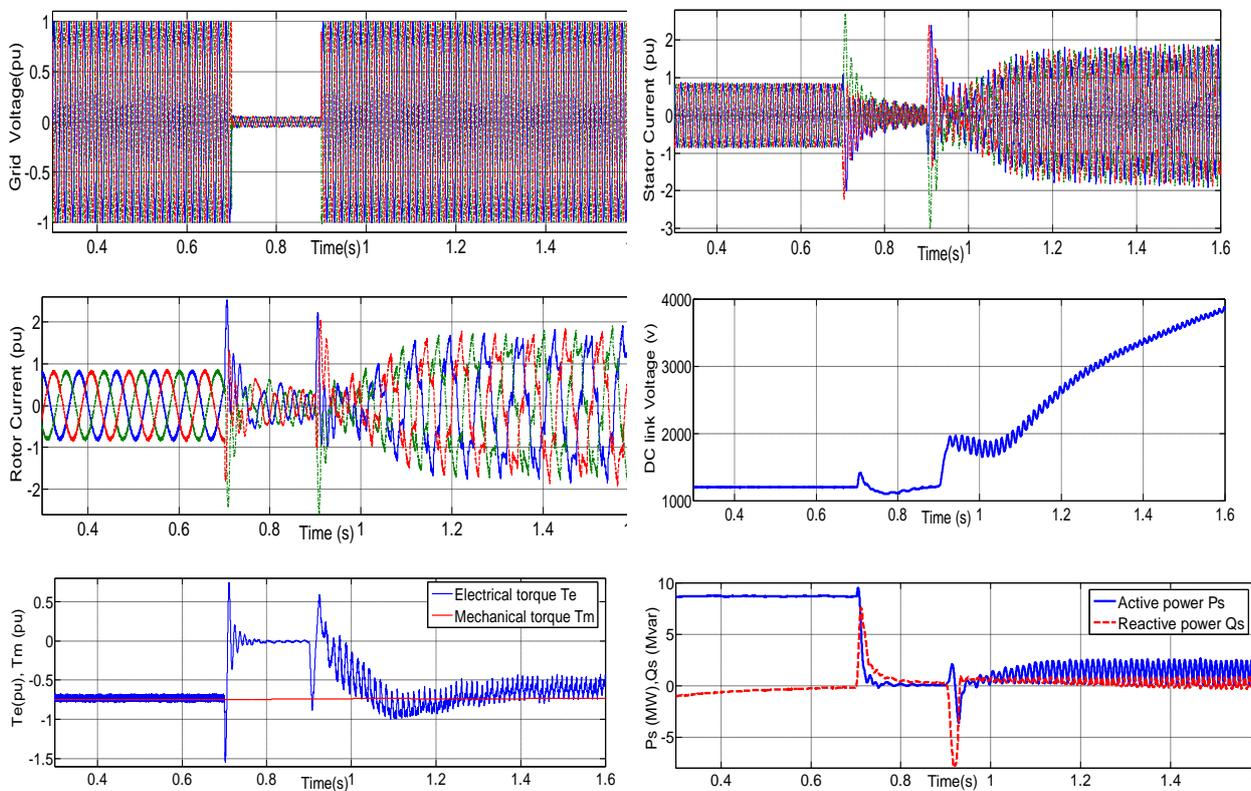
Fig. 3: Three-phase 0.95pu voltage dip for 0.2s
