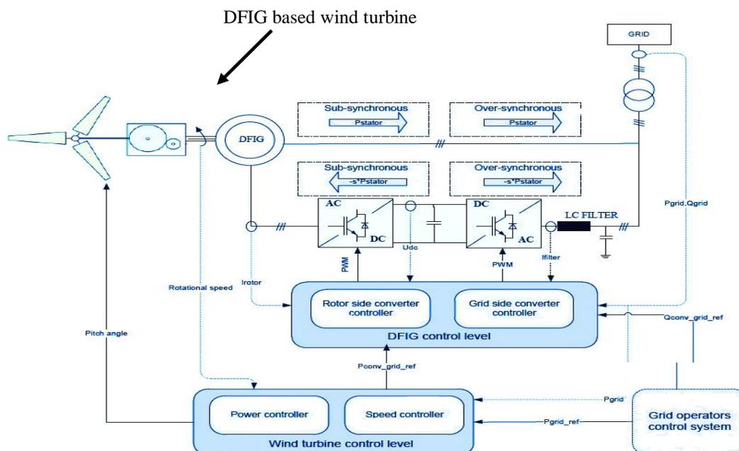
Fig. 1: Block diagram for a wind turbine control based on DFIG [36].
