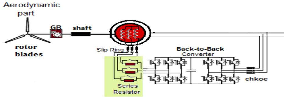
Fig. 5: DFIG based system extended by Series Resistor Protection Scheme
