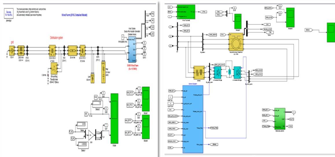
Fig. A1 Matlab/Simulink model of the DFIG based wind turbine
