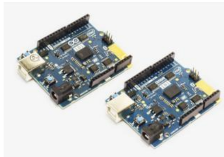
Figure 5: Two types of Arduino (USA on left, Outside USA on right) with Intel curie microcontroller
