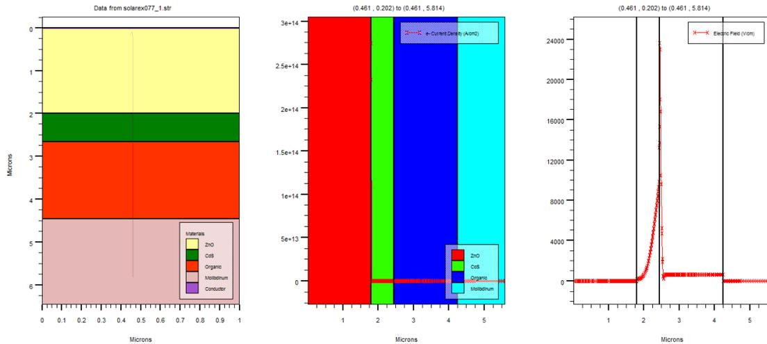
**Fig2.** Configuration, current density and electric field of the P3HT/CdSe solar cells with  $10^{16} \text{cm}^{-3}$  for doping in electron donor.
