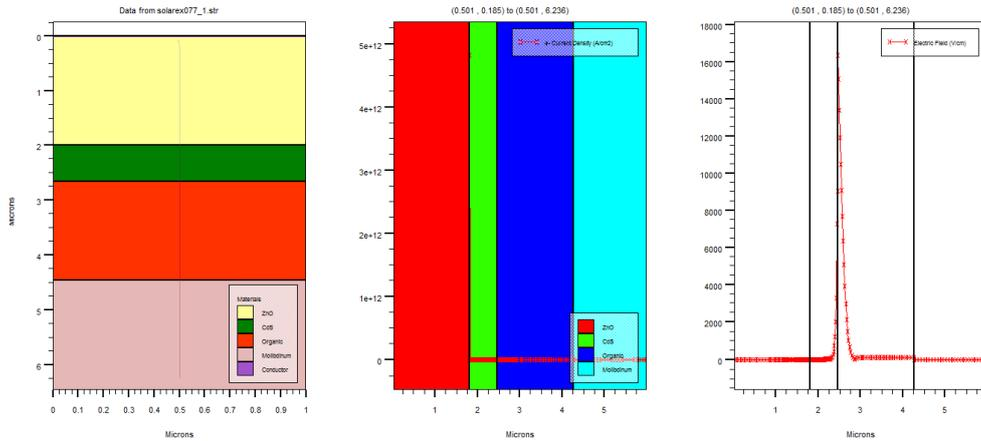
**Fig6.** Configuration, current density and electric field of the P3HT/CdSe solar cells with doping  $1.6 \times 10^{15} \text{ cm}^{-3}$  in hole donor.
