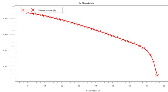
**Fig3.** Current- voltage curve of the P3HT/CdSe solar cells with doping  $10^{16} \text{cm}^{-3}$  in electron donor.
