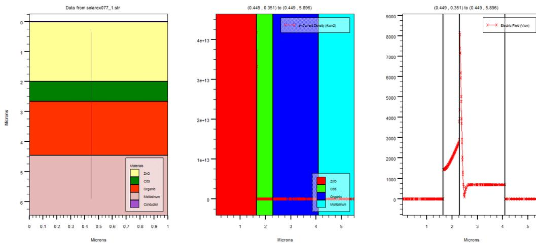
**Fig4.** Configuration, current density and electric field of the P3HT/CdSe solar cells with doping  $1.6 \times 10^{13} \text{ cm}^{-3}$  in hole donor.
