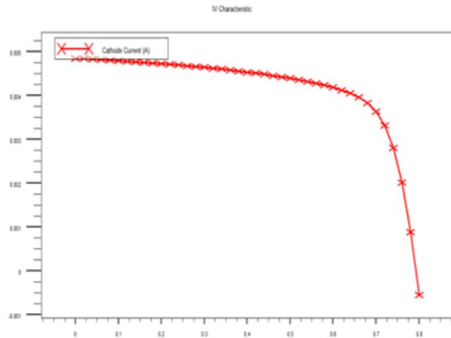
**Fig3.** Current- voltage curve of the P3HT/CdSe solar cells with doping  $1.6 \times 10^{13} \text{ cm}^{-3}$  in hole donor.
