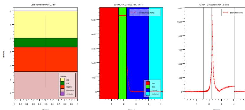
**Fig1.** Configuration, current density and electric field of the P3HT/CdSe solar cells with  $10^{13} \text{ cm}^{-3}$  for doping in electron donor.
