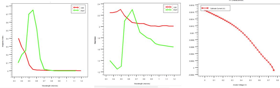
**Fig5.** Refractive index and current-voltage curve of the P3HT/CdSe solar cells with doping  $13 \times 10^{14} \text{ cm}^{-3}$  and  $16 \times 10^{14} \text{ cm}^{-3}$  in electron donor and hole donor, respectively.
