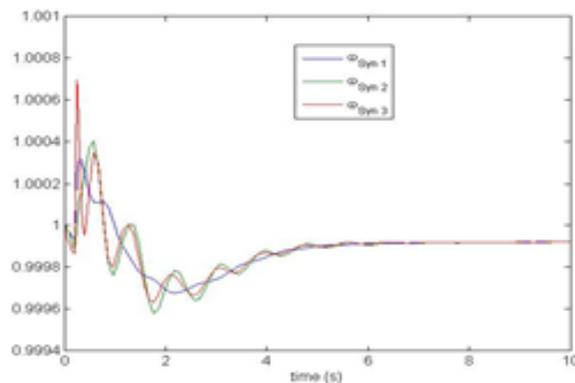
Figure(8) Speed variations of Synchronous Generators with STATCOM at Bus -2.
