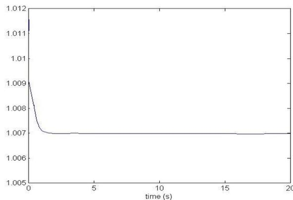
**Fig(14)** Plot of Bus-1 voltage with STATCOM
