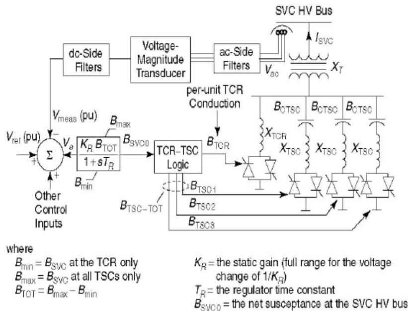
Fig(1) Functional Diagram of SVC
