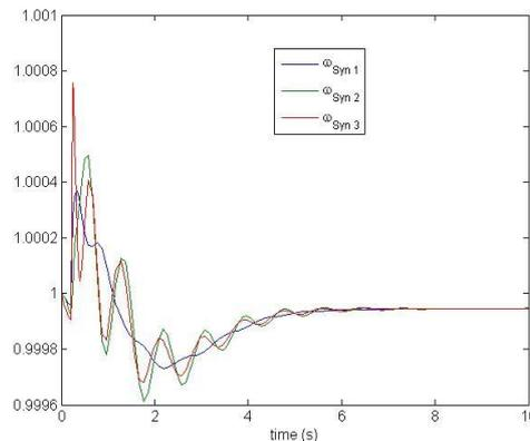
Fig (9) Speed variations of Synchronous Generators with SVC at Bus -2.
