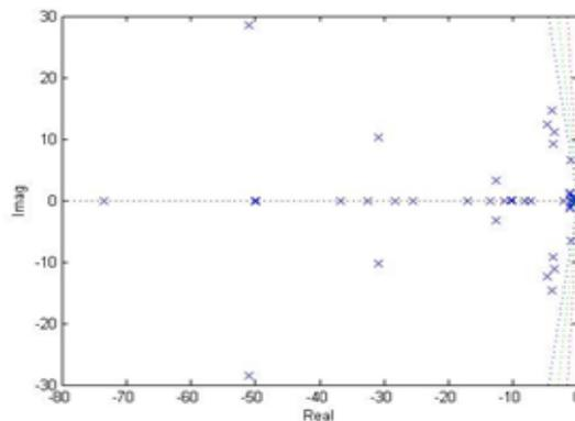
**Fig(10)** Eigenvalues plot with STATCOM
