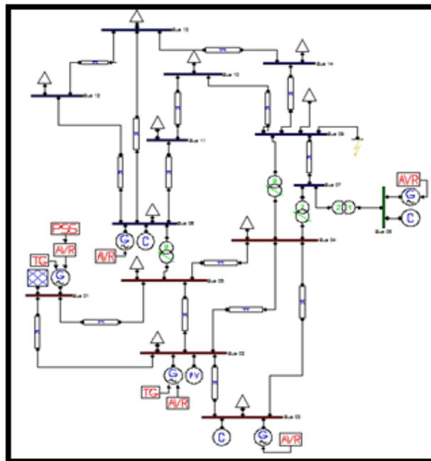
Fig (3) Model of IEEE 14 Bus system
