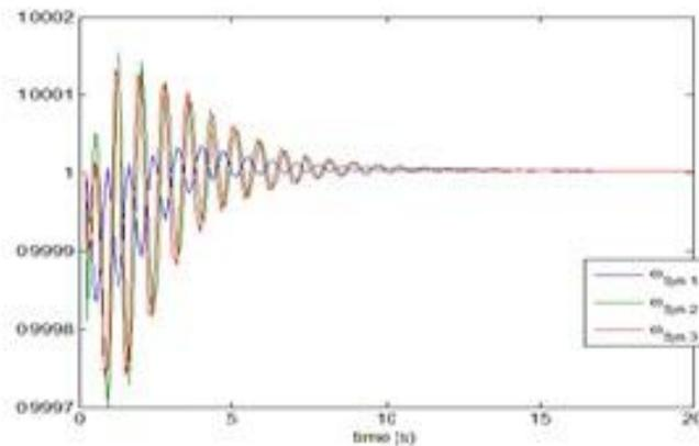
**Fig(5)** Speed variations of Synchronous Generators without PSS.
