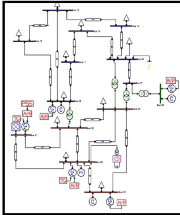
Figure(7) IEEE 14 Bus with STATCOM at Bus-2
