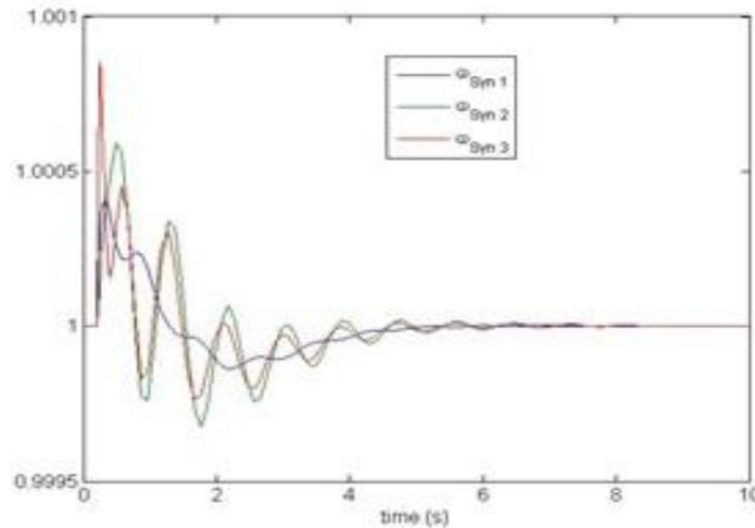
**Fig(4)** Speed variations of Synchronous Generators with PSS.
