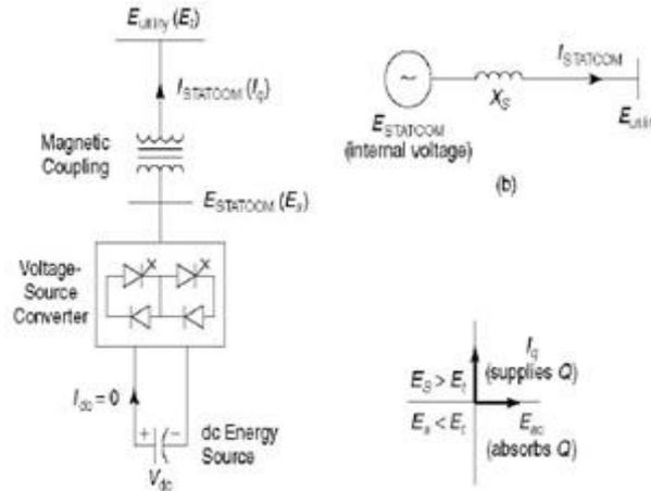
Fig(2) Basic STATCOM Principle Diagram
