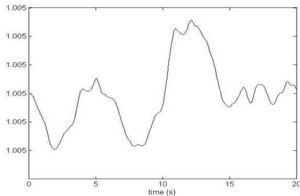
**Fig(13)** Plot of Bus-1 voltage without STATCOM
