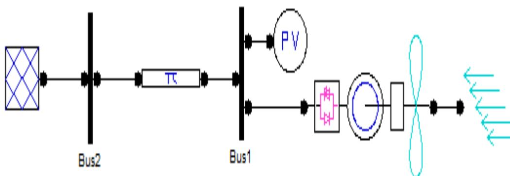
**Fig(12)** Variable speed wind turbine with direct drive synchronous generator.
