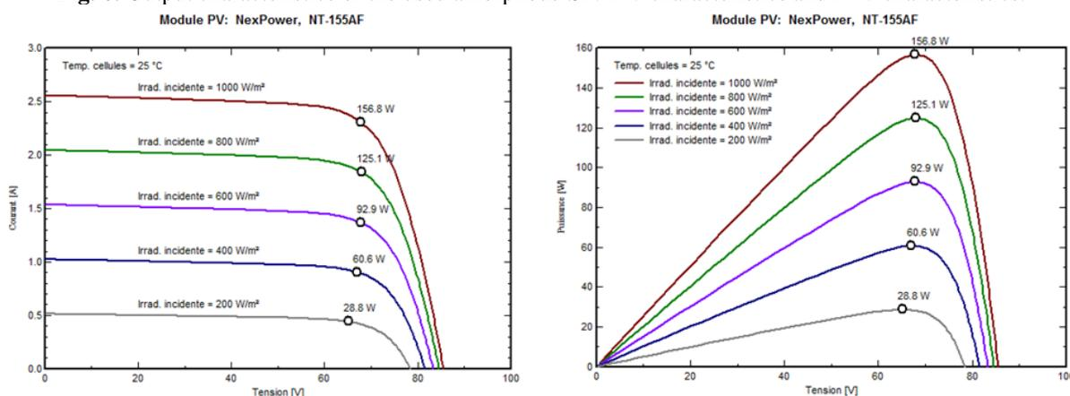
**Fig. 7.** Output characteristics of the used polycrystalline-Si : I-V characteristics and P-V characteristics.
