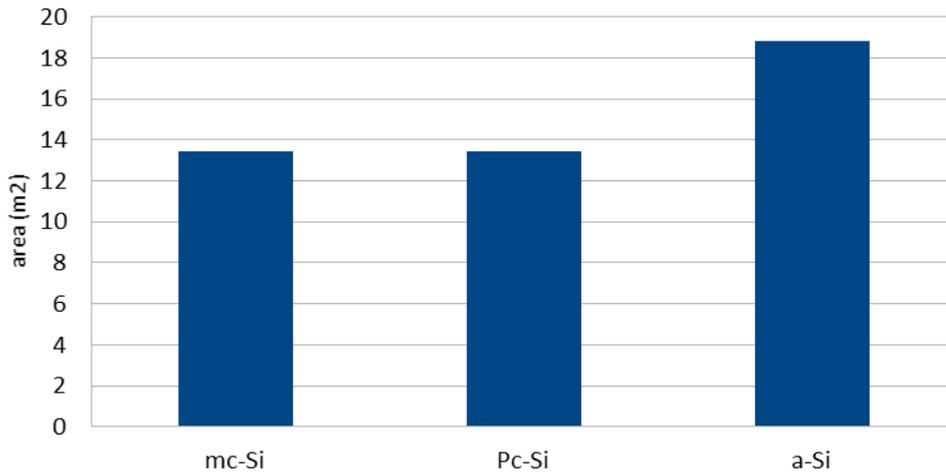
**Fig.10.** Comparison of the areas occupied by each power system.
