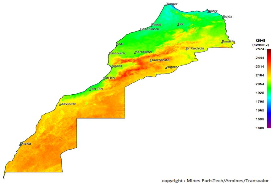
**Fig.1.**Map of global horizontal solar irradiation in Morocco
