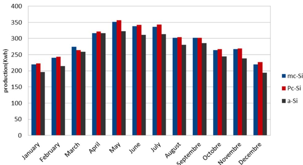
Fig.8. Harvested energy profile from the three-plant all year round.
