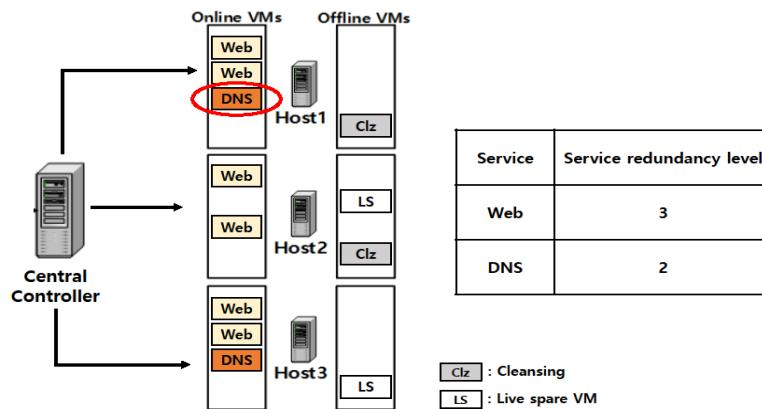
**Fig. 7:** An example of a system with three hosts and each host has four VMs
