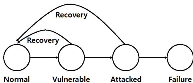
**Fig. 3:** SCIT state transition diagram [8]
