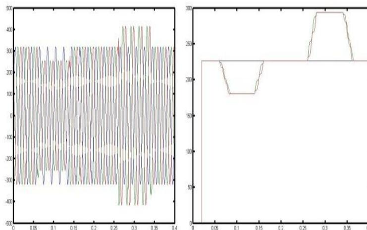
**Fig.15.** Simulated wave form showing sag and swell in phase B and C
