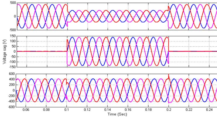
Fig.24. Simulated wave form showing sag in all three phases of power system, DVR voltage and load voltage
