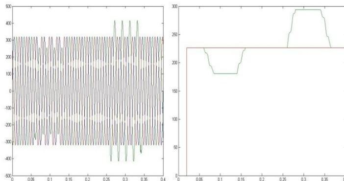
Fig.9. Simulated wave form showing sag and swell in phase-B
