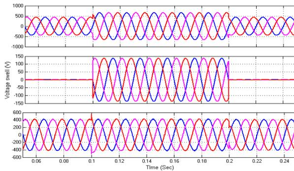
Fig.25. Simulated wave form showing swell in all three phases of power system, DVR voltage and load voltage
