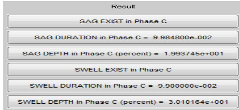
Fig.10. Result showing existence of sag and swell in phase-C
