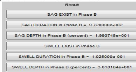
Fig.8. Result showing existence of sag and swell in phase-B
