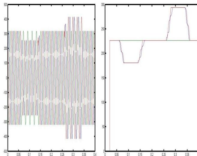
Fig.17. Simulated wave form showing sag and swell in phase A and C
