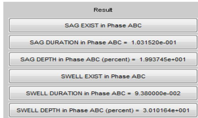
Fig.18. Result showing existence of sag and swell in all three phases
