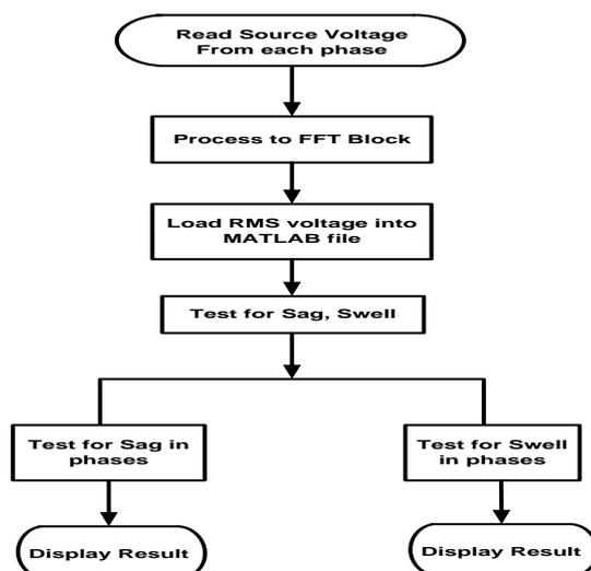
Fig.3. Flow chart for Fault Identification using FFT analysis
