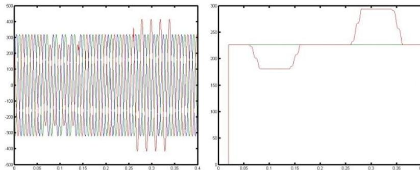
Fig.11. Simulated wave form showing sag and swell in phase-C
