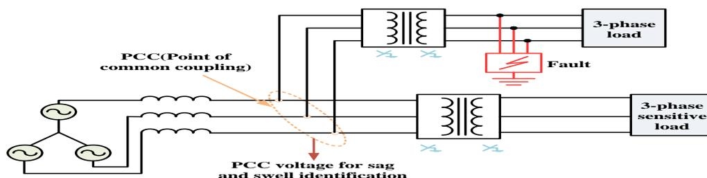
Fig.1. Power system network schematic arrangement with presence of fault
