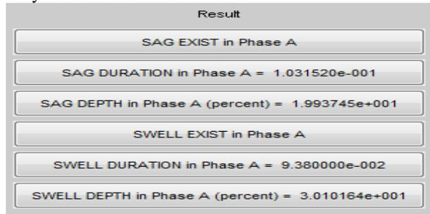
Fig.6. Result showing existence of sag and swell in phase-A
