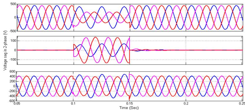
**Fig.22.** Simulated wave form showing sag in two phases of power system, DVR voltage and load voltage
