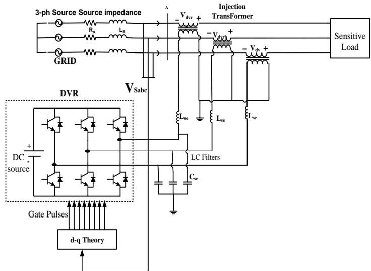
Fig.5. Schematic arrangement of complete power system with d-q control for DVR
