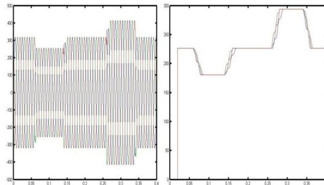
Fig.19. Simulated wave form showing sag and swell in all three phases
