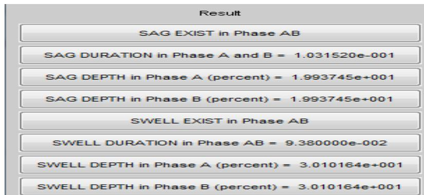
Fig.12. Result showing existence of sag and swell in phase-A and B
