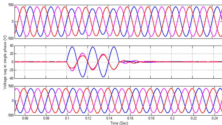
Fig.20. Simulated wave form showing sag in one phase of power system, DVR voltage and load voltage
