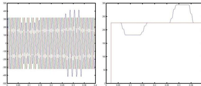
Fig.7. Simulated wave form showing sag and swell in one phase
