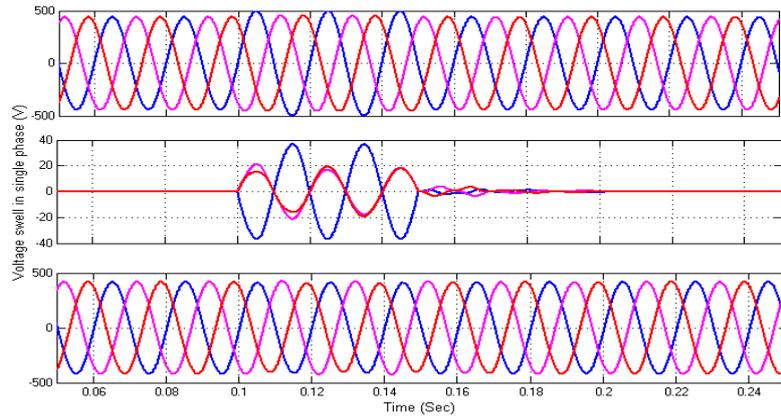
**Fig.21.** Simulated wave form showing swell in one phase of power system, DVR voltage and load voltage
