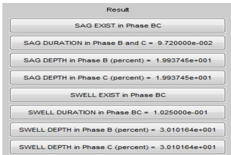
**Fig.14.** Result showing existence of sag and swell in phase B and C
