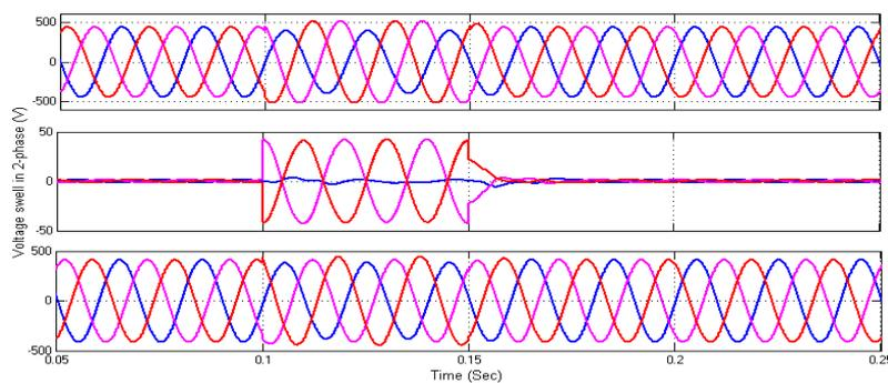
**Fig.23.** Simulated wave form showing swell in two phases of power system, DVR voltage and load voltage
