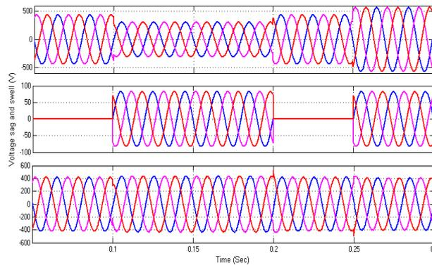
Fig.26. Simulated wave form showing sag and swell existence in all three phases of power system, DVR voltage and load voltage
