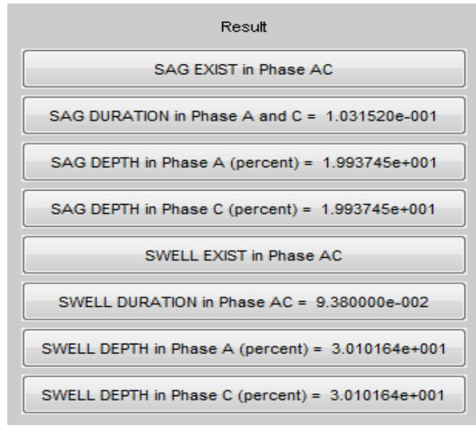
Fig.16. Result showing existence of sag and swell in phase-A and C
