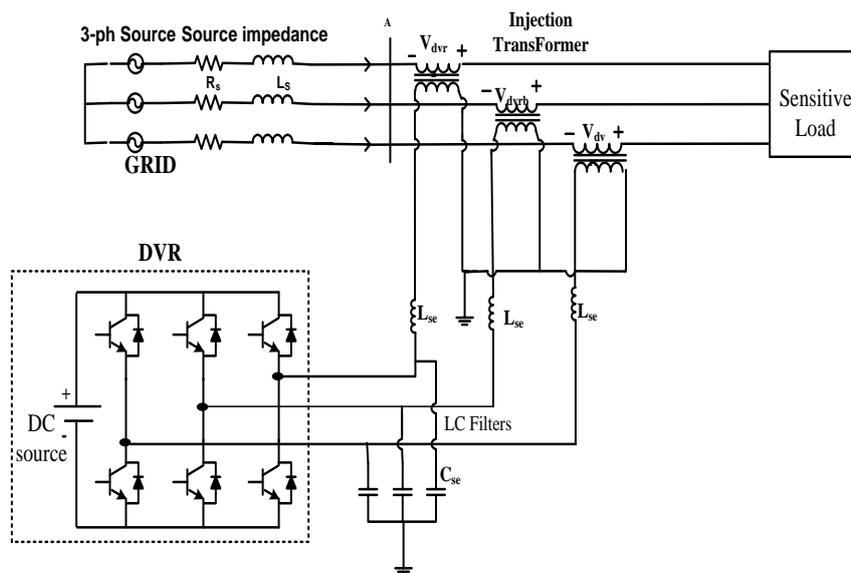
Fig.2. Schematic arrangement of power system for voltage problem mitigation with DVR
