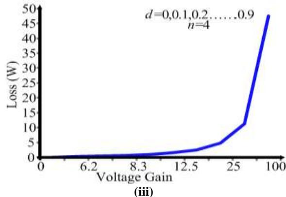
Fig. 8 (i) Efficiency versus load curve for the proposed dc-dc converter and comparison with existing versions; (ii) Loss versus gain plot by varying voltage gain with the variation of turns ratio ( $n$ ), keeping duty cycle ( $d$ ) constant; (iii) Loss versus gain plot by varying voltage gain with the variation of  $d$ , keeping  $n$  constant.
