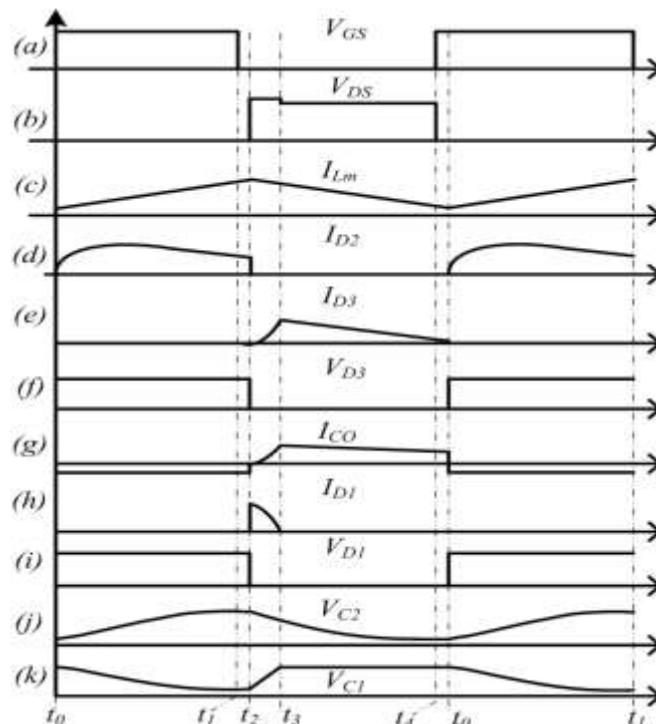
**Fig. 5** Typical waveforms during CCM operation.
