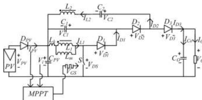
Fig 1. Circuit topology of dc/dc converter
