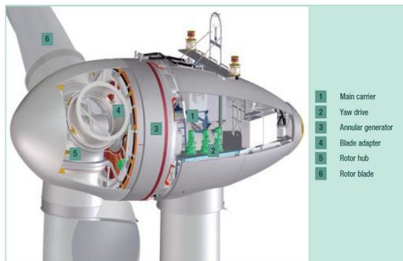
**Fig.1:** Cross Sectional view of Wind Generator
