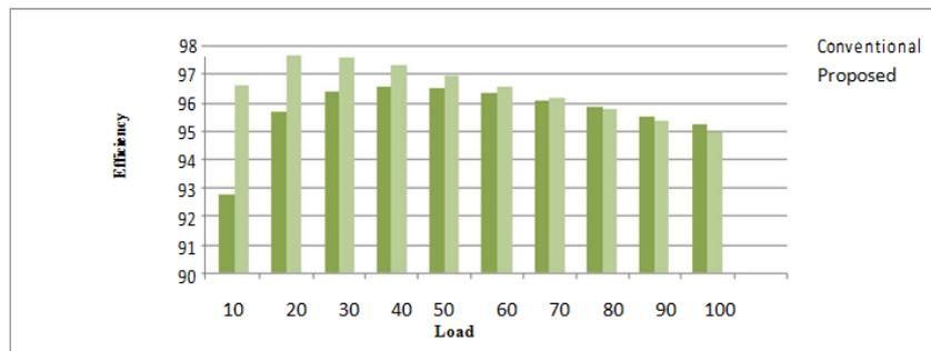
**Fig. 4(b).** Comparison of conventional and proposed circuit, Efficiency verses load
