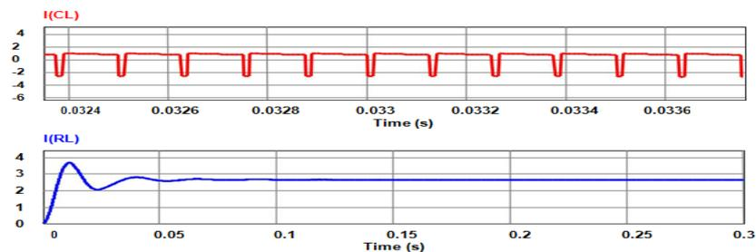
Fig. 3(d). Currents through capacitor  $CL$  & resistor  $RL$
