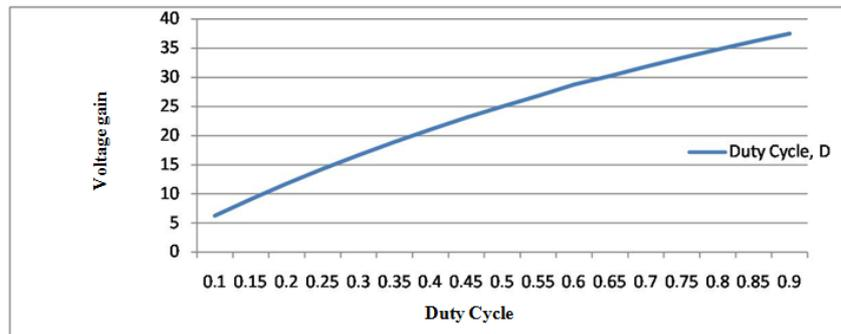
**Fig. 5.** Voltage gain of the proposed circuit throughout the duty cycle 0.1 to 0.9
