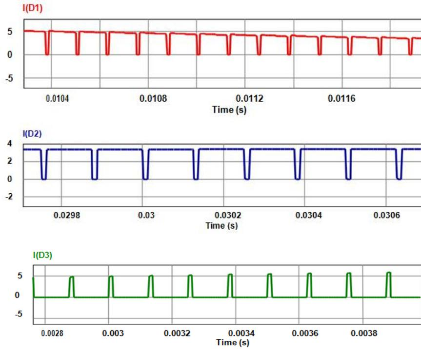
Fig. 3(b). Currents through diodes  $D1$ ,  $D2$  &  $D3$
