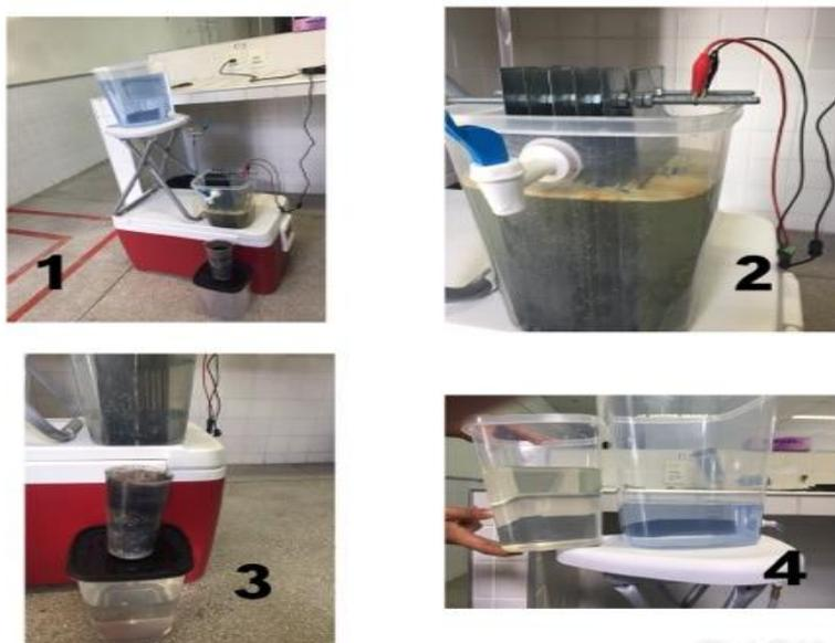
**Figure 3**- Purification of textile effluent at continuous flow. 1- electroflocculation reactor assembly with continuous flow, 2- electroflocculation reactor, 3 fixed-bed filter, 4-comparison of raw and treated effluent.
