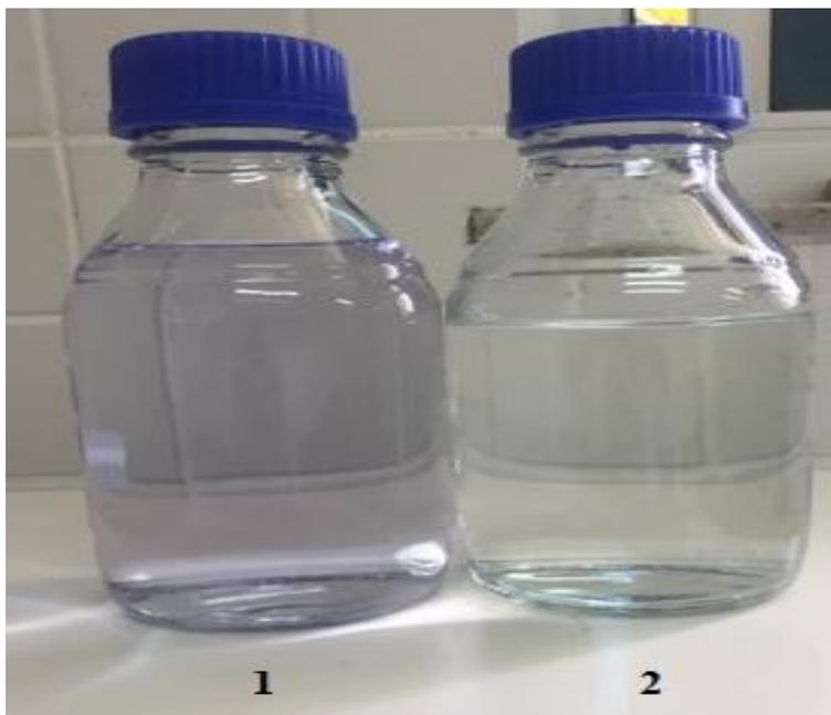
**Figure 6** - Textile effluent. (1) - before electroflocculation, (2) - after electroflocculation.
