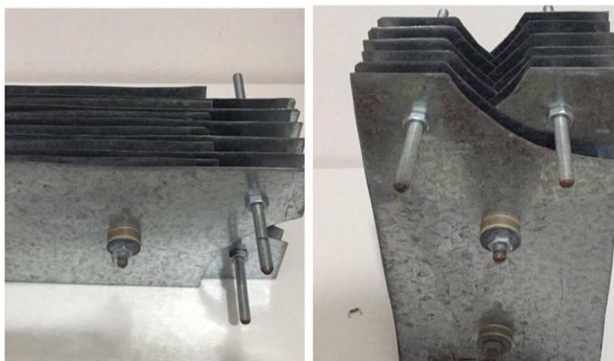
**Figure 2** - Monopolar plates arrangement connected in parallel.
