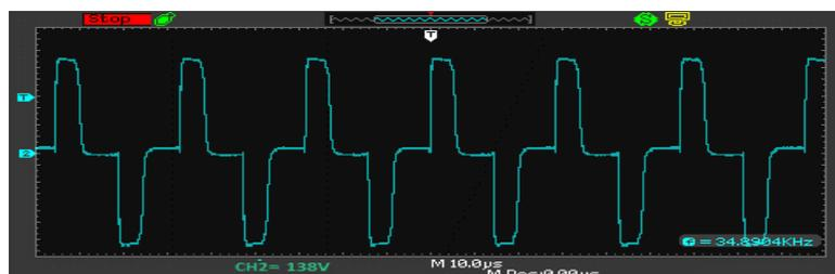
Fig 28 Output across load for R5= 800ohm
