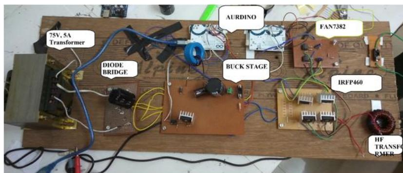
Fig 11 Hardware implementation diagram
