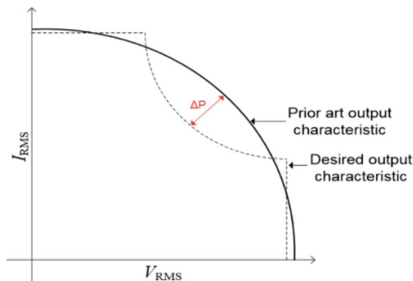
Fig 2 Output characteristics of resonant inverter
