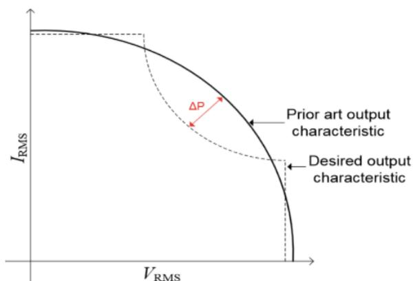
Fig 2 Output characteristics of resonant inverter
