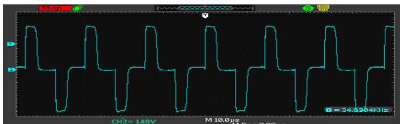
Fig 28 Output across load for R6= 940ohm
