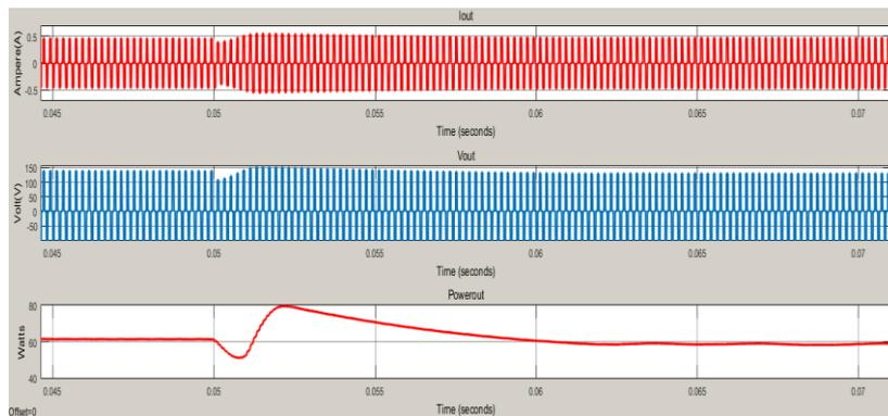
Fig 6 Output in constant current mode
