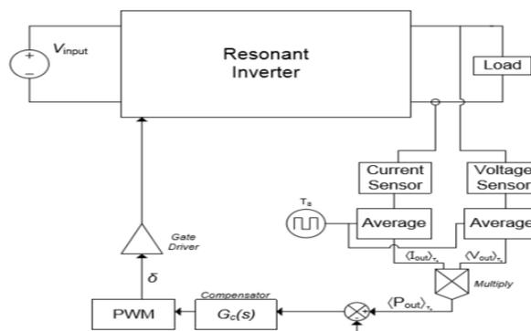
Fig 3 Closed loop control of resonant inverter [3]
