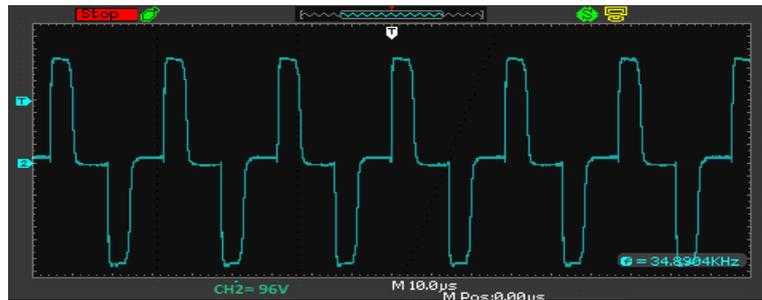
Fig 28 Output across load for R1= 470ohm
