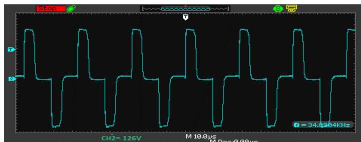
Fig 28 Output across load for R3= 673ohm
