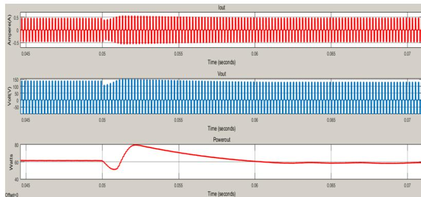
Fig 6 Output in constant current mode
