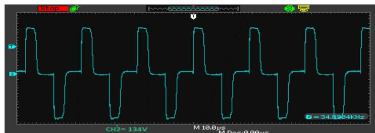
Fig 28 Output across load for R4= 770ohm
