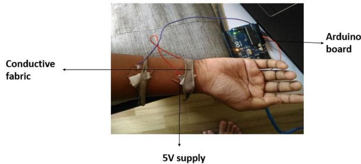
Fig 9 Experimental setup of skin resistance measurement
