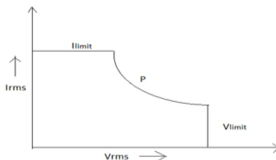
Fig 1 Power characteristics
