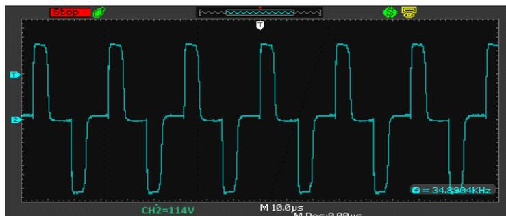
Fig 28 Output across load for R2= 560ohm
