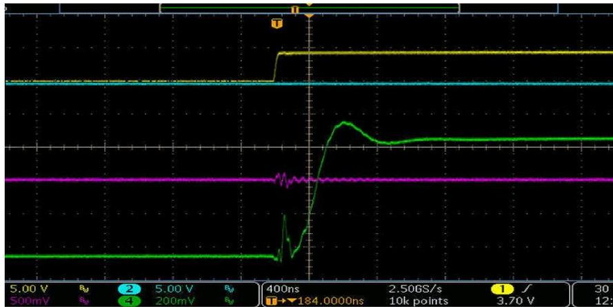
Fig .4Oscilloscope traces: yellow trace is anintegrating gate signal; purple trace is input signal; green trace is output signal
